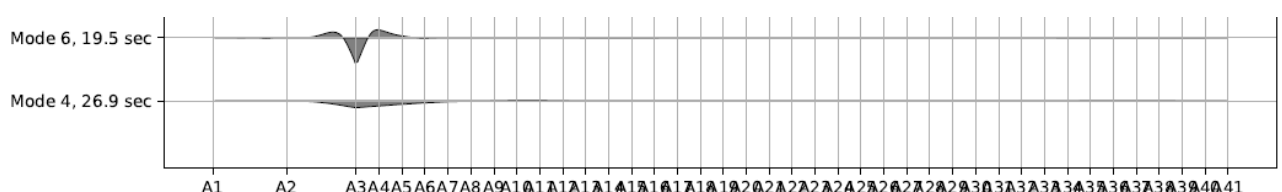
Figure 3-9 Pendulum mode (mode 6) when axis A3 is drydocked.
