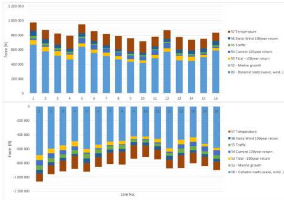
> Figure 13-5 Load components in mooring line
