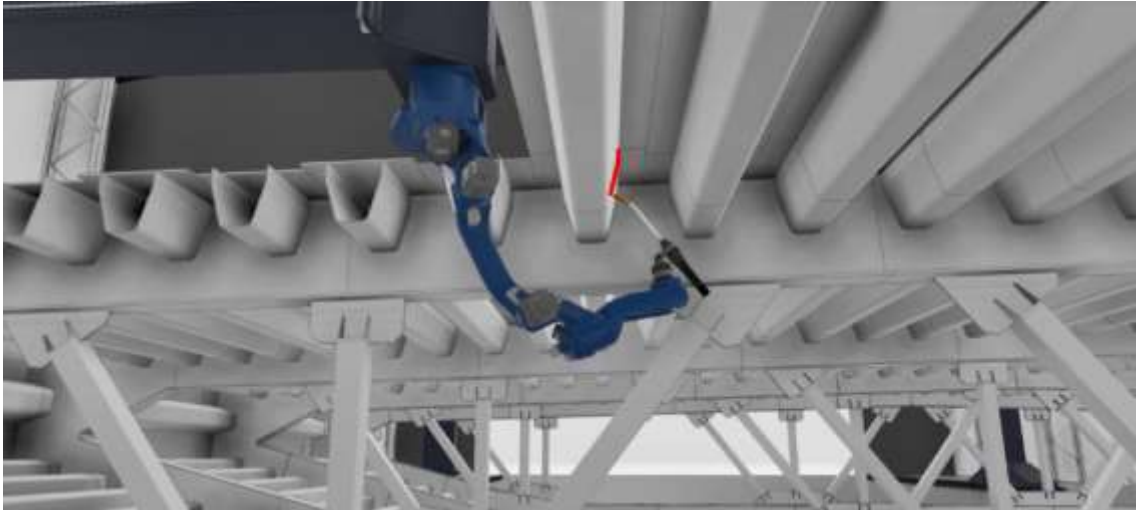
> Figure 18-17: Welding of longitudinal stiffeners
