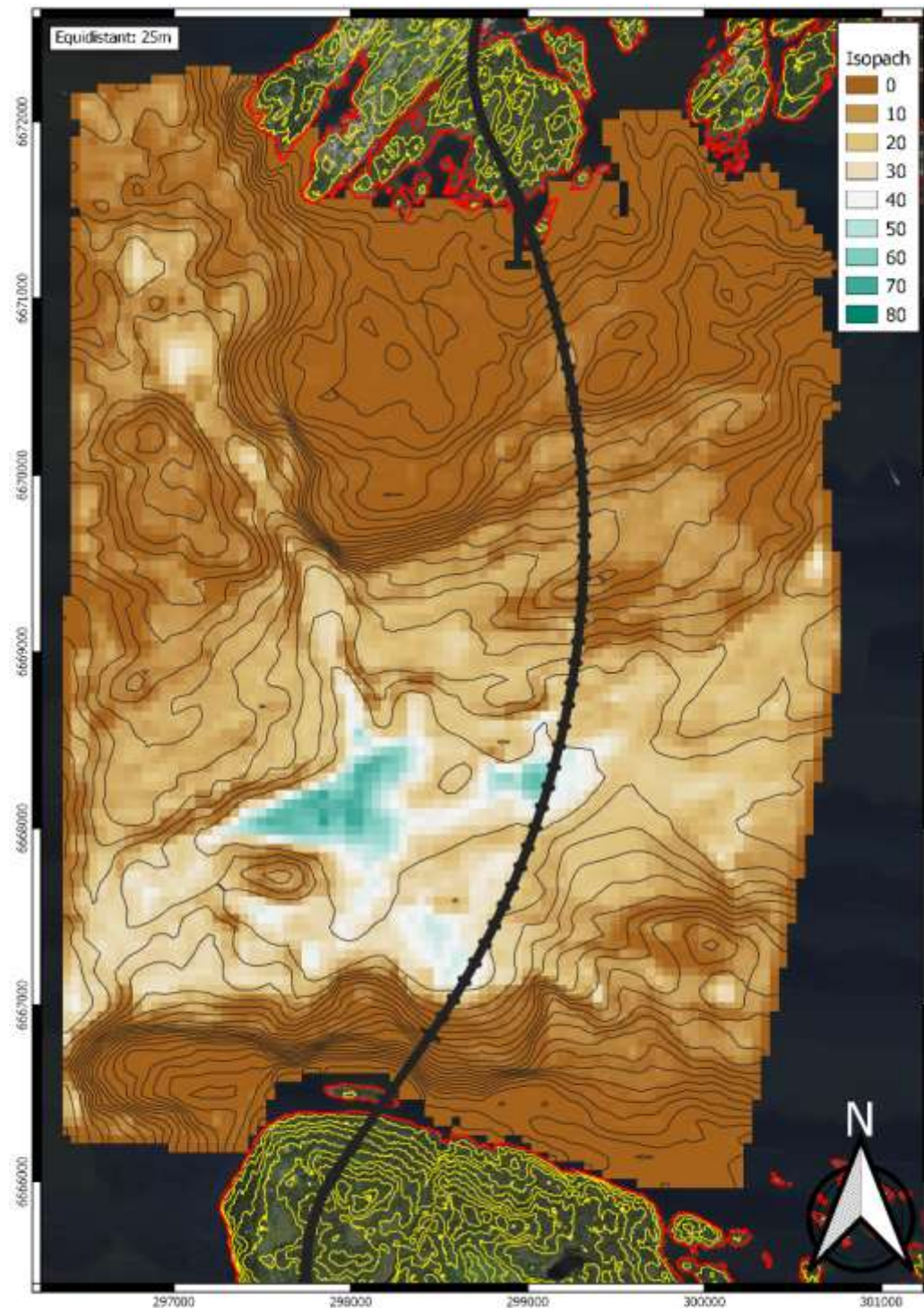
> Figure 14-2 - Interpolated isopach from data provided by DOF 2016 and 2018 shown together with proposed anchor locations.
