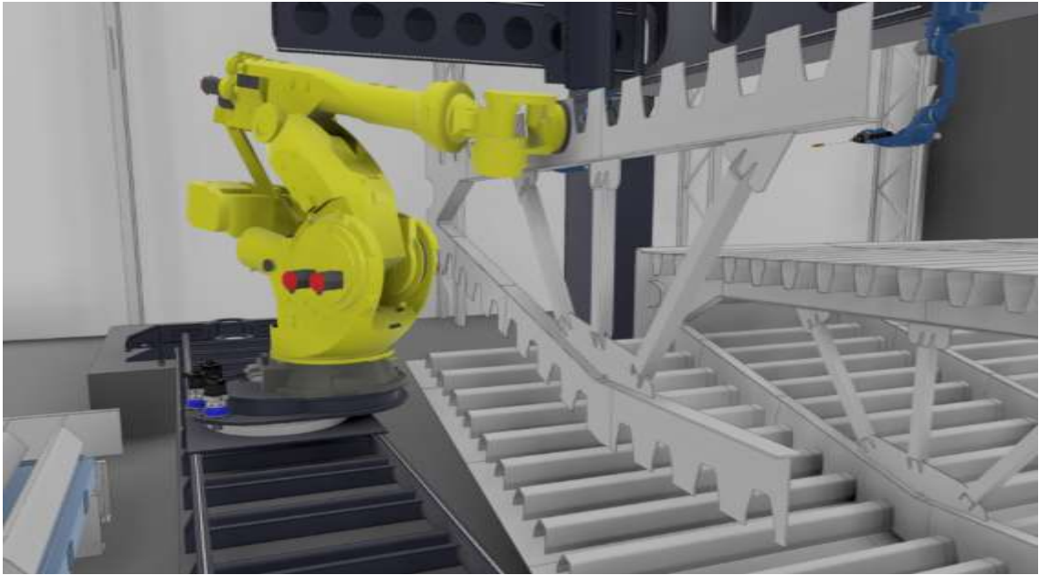
> Figure 18-14: Robot mounting of transverse girder
