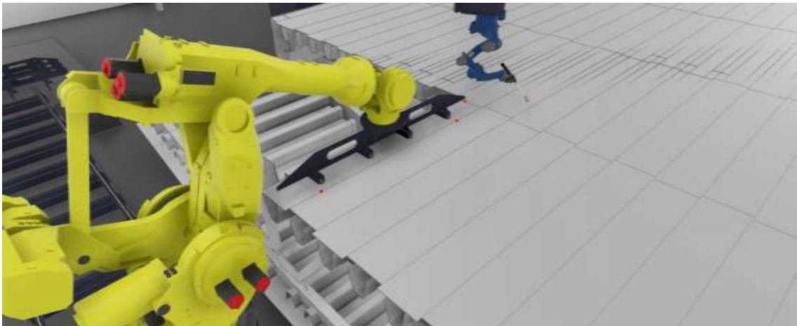
> Figure 18-16: Mounting of top plate elements
