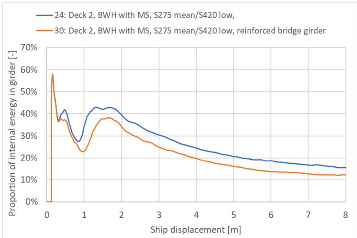
> Figure 5-4 Proportion of internal energy in girder [-] impact deckhouse-girder, sensitivity of girder cross section
