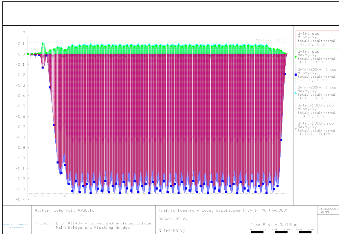
Figure 3-17 Traffic loading, vertical deformation in bridge girder – comparison of envelope values for load length dependent traffic loading and infinite loaded length with 200m load intensity and 1000m load intensity.
