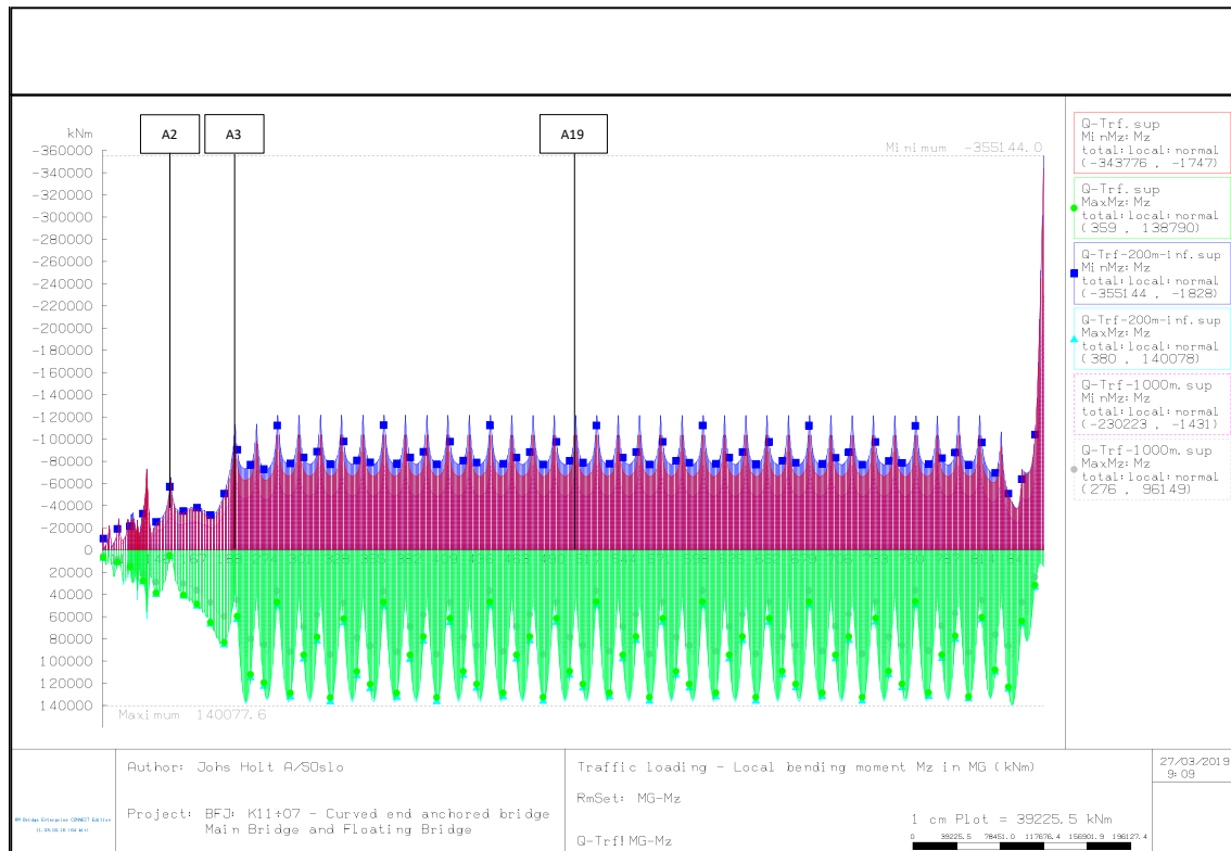
Figure 3-10 Traffic loading, weak axis bending moment – comparison of envelope values for load length dependent traffic loading and infinite loaded length with 200m load intensity and 1000m load intensity.
