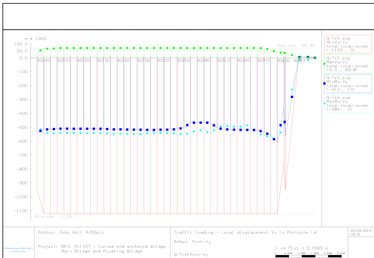
Figure 3-19 Traffic loading, vertical deformation in pontoons – envelope values for load length dependent traffic sorted on Min/Max Vertical deformation and the Vertical deformation associated with Min/Max Roll
