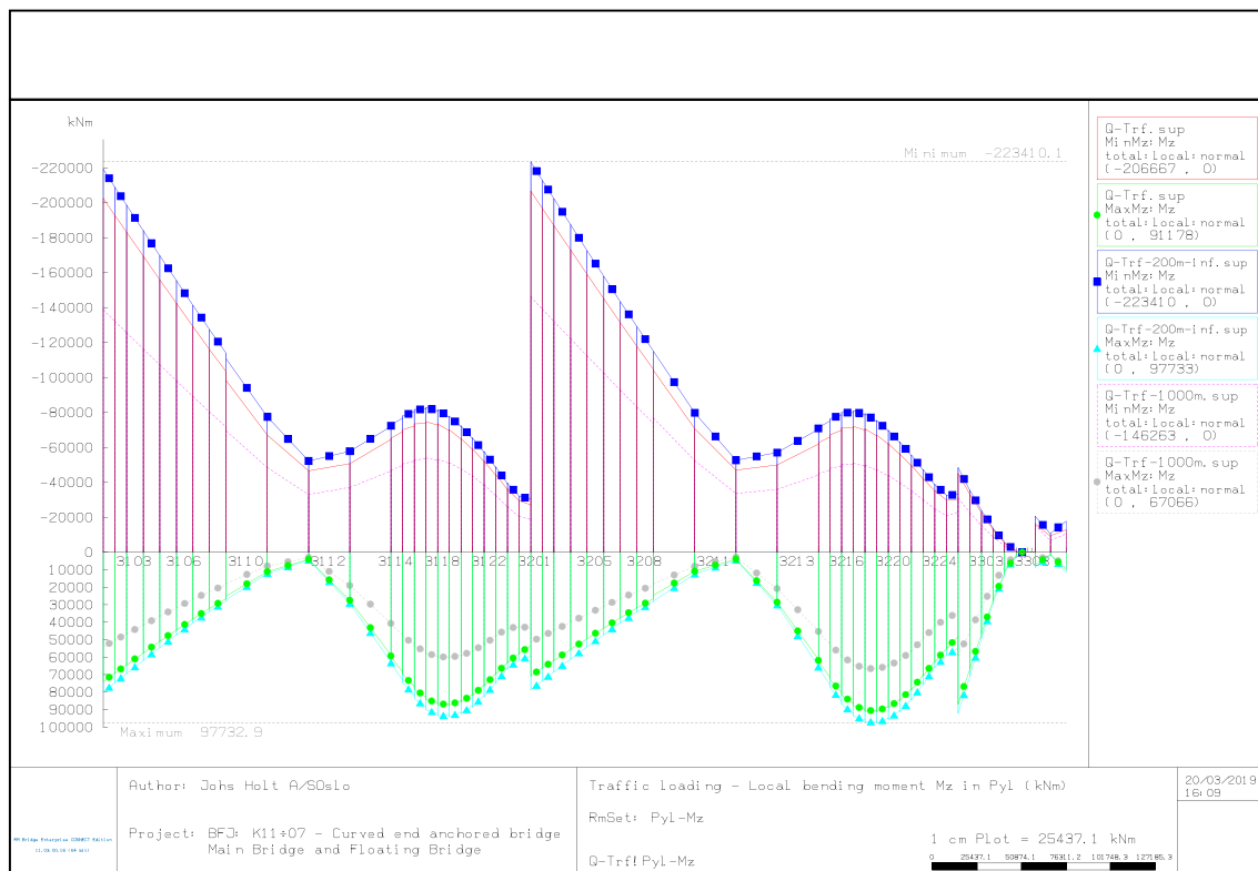
Figure 3-14 Traffic loading, bending moment about transverse bridge axis in west pylon leg and spire – comparison of envelope values for load length dependent traffic loading and infinite loaded length with 200m load intensity and 1000m load intensity.
