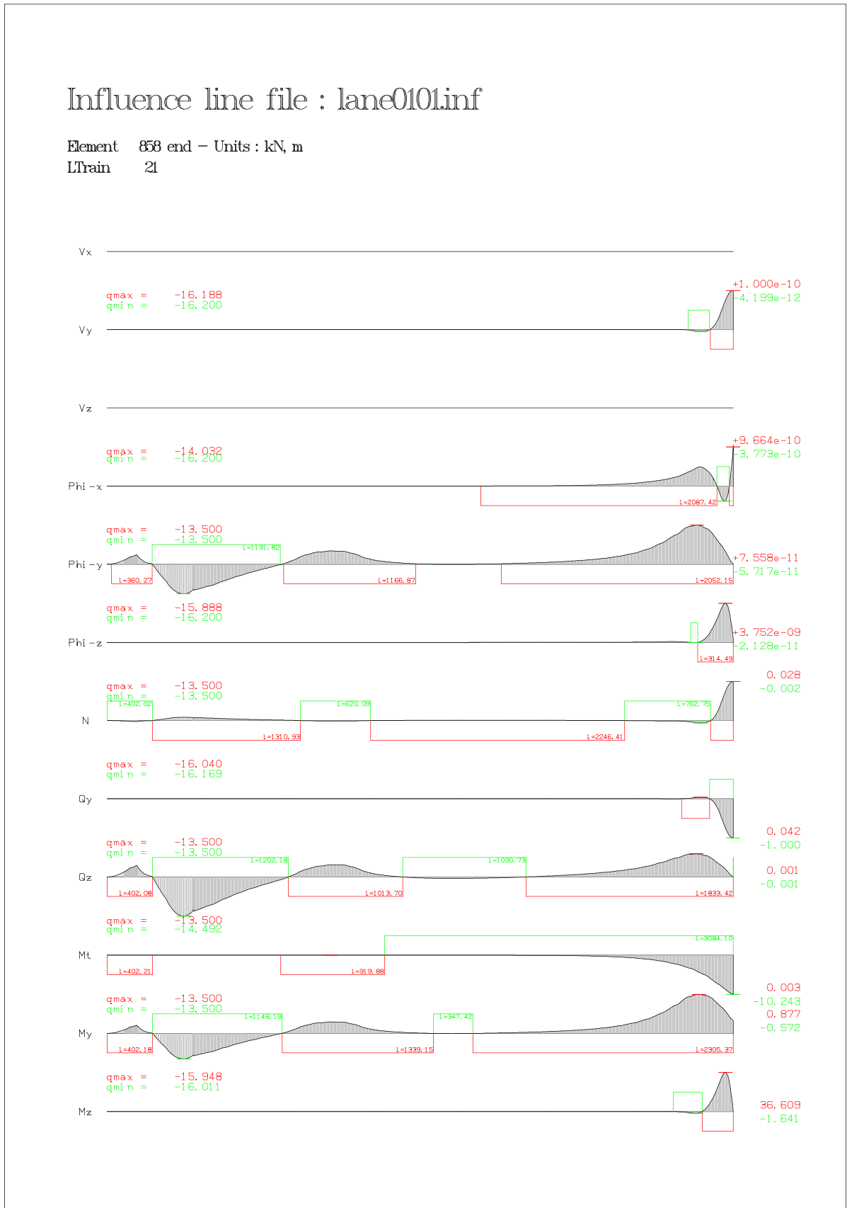
Figure 3-6 Influence lines for lane 1, load train 21 – Bridge girder support section at axis 41 (north abutment)
