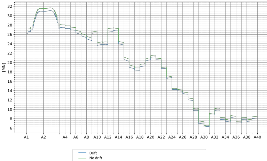
Figure 8-20 Comparison of Axial force for simulations with and without second order drift
