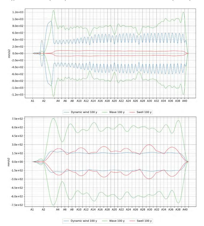
Figure 4-12 Overview of contributions to vertical (top) and transverse (bottom) acceleration from wave and wind load components for the K12\_07 concept, 100 year return period.
