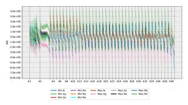
Figure 3-12 Traffic loads – vertical shear force in bridge girder (envelope values) [MN]
