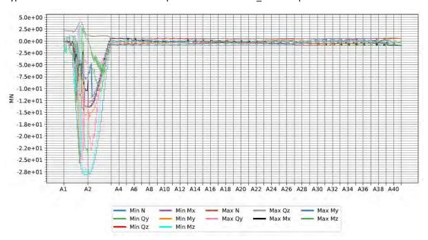
Figure 3-10 Traffic loads – Axial force in bridge girder (envelope values) [MN]
