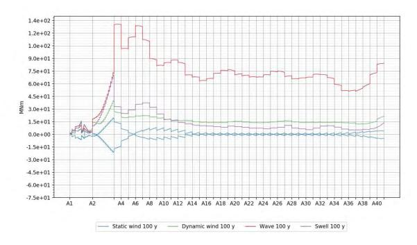
Figure 4-5 Overview of torsional moment contribution from slowly varying loads (top) and wave and wind loading (bottom) for the K12\_07 concept.
