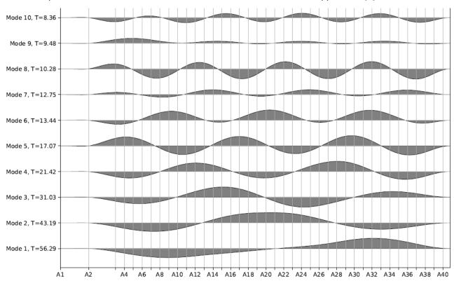
Figure 4-1 Orcaflex transverse eigenmodes for K12\_07
