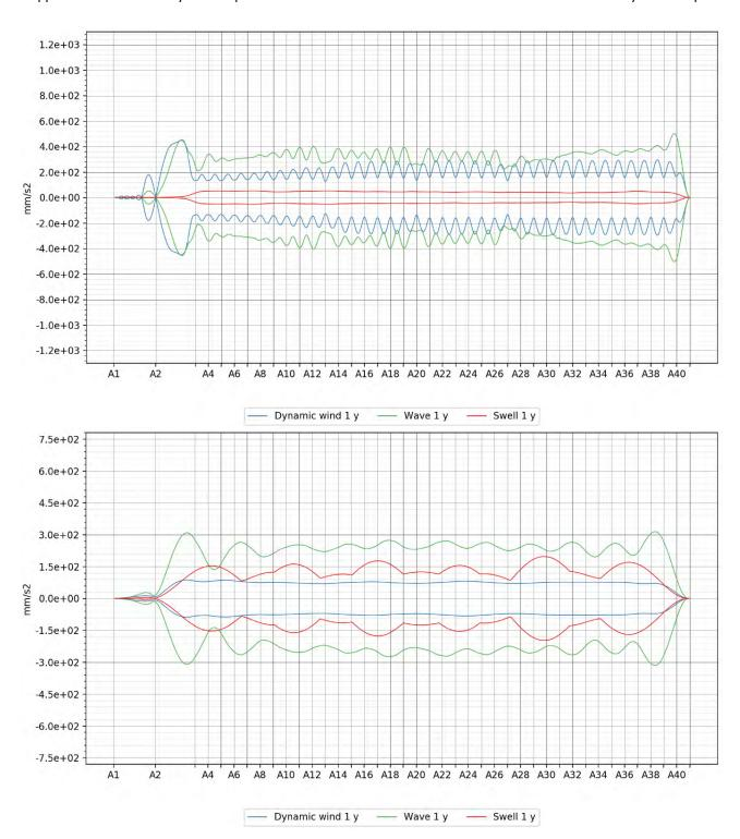
Figure 4-16 Overview of contributions to vertical (top) and transverse (bottom) acceleration from wave and wind load components for the K12\_07 concept, 1 year return period.
