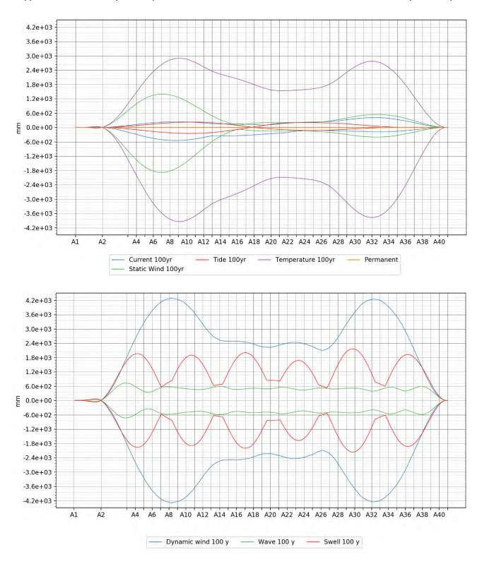
Figure 4-9 Overview of contributions to transverse displacements from slowly varying (top) and wave and wind (bottom) load components for the K12\_07 concept, 100 year return period.
