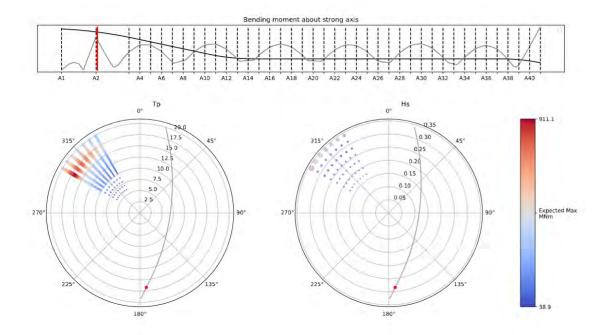
Figure 2-3: Bending moment about strong axis in the bridge girder at the tower for 100-year return period swell sea states.
