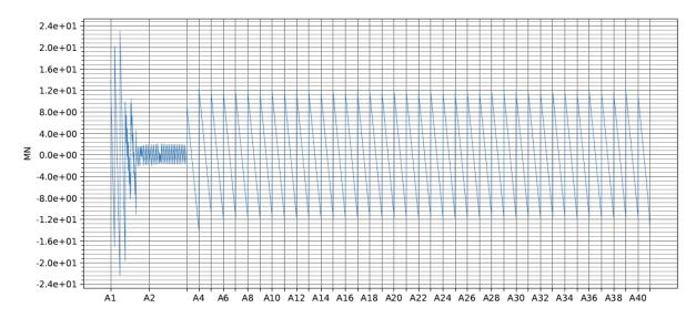
Figure 3-2 Permanent loads – vertical shear force in bridge girder [MN]
