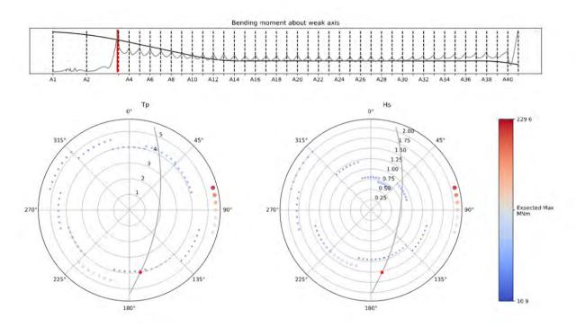
Figure 2-1: 100 year return period wind sea, 1 hour maximum bending moment about weak axis
