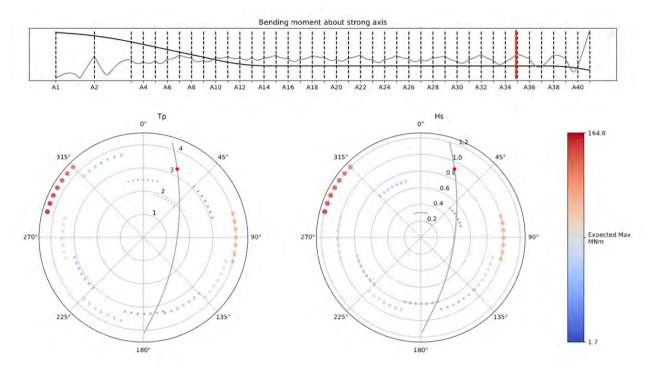
Figure 2-2: 1 year return period wind sea, 1 hour maximum bending moment about strong axis
