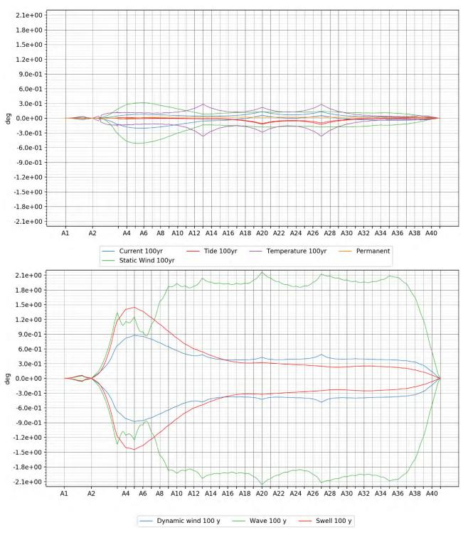
Figure 4-11 Overview of contributions to rotation about the longitudinal bridge axis from slowly varying (top) and wave and wind (bottom) load components for the K12\_07 concept, 100 year return period.
