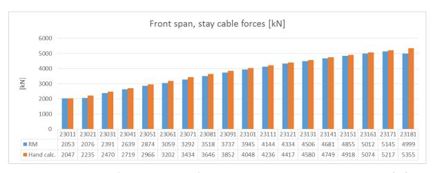
Figure 3-6 Permanent loads, front span stay cable forces – comparison RM Bridge to hand calculations [kN]
