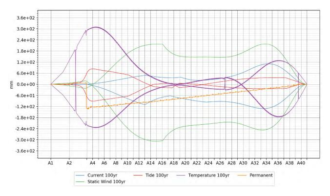
Figure 4-8 Overview of contributions to longitudinal displacements from various load components for the K12\_07 concept, 100 year return period.
