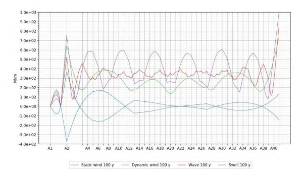
Figure 4-3 Overview of strong-axis bending moment contribution from slowly varying loads (top) and wave and wind loading (bottom) for the K12\_07 concept.
