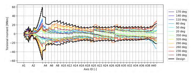
Figure 2-6 Wind-screening, torsional moment for K12\_06
