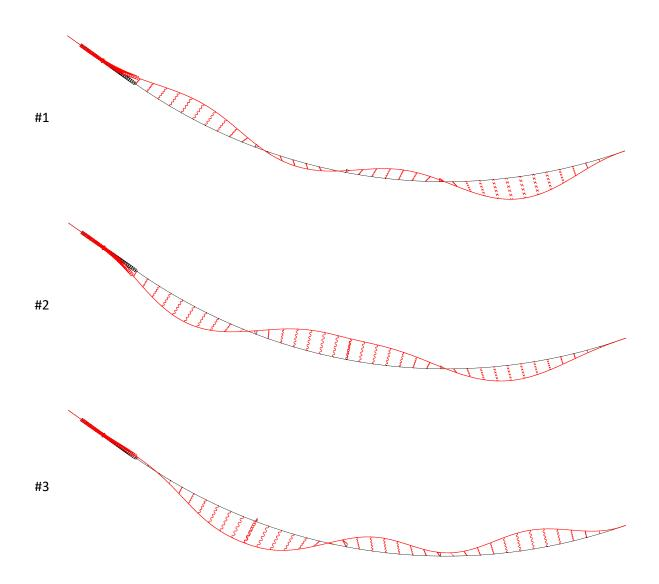
Figure 3-15 First three buckling modes of K12
