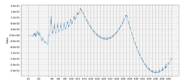
Figure 3-4 Permanent loads - Strong-axis bending moment in bridge girder for K12\_07 [MNm]
