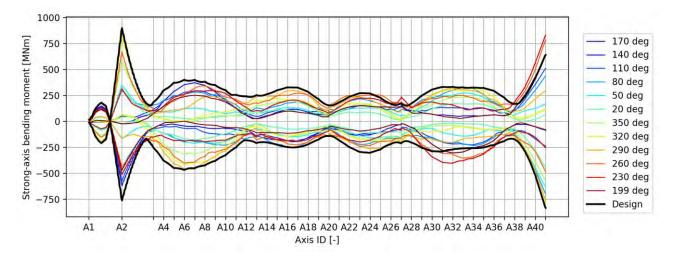
Figure 2-5 Wind-screening, strong-axis bending moment for K12\_06
