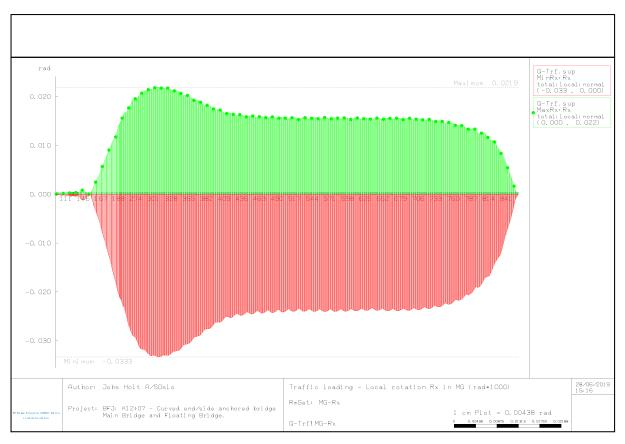
Figure 3-14 Traffic loading – rotation (roll) in bridge girder (envelope values) [rad]
