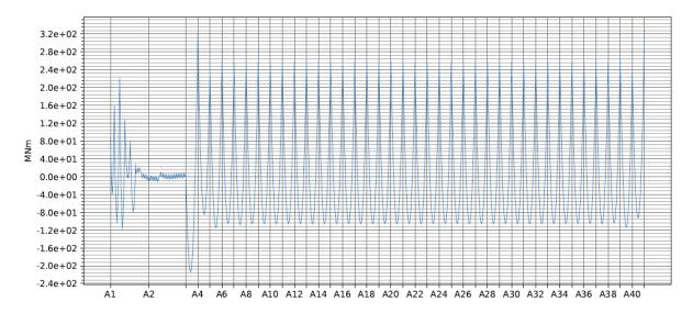
Figure 3-3 Permanent loads – Weak axis bending moment in bridge girder for K11\_07 [MNm]
