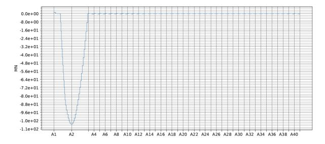
Figure 3-1 Permanent loads – Axial force in bridge girder [MN]
