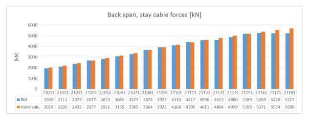
Figure 3-5 Permanent loads, back span stay cable forces – comparison RM Bridge to hand calculations [kN]
