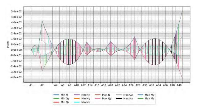
Figure 3-9 Temperature loads – Strong axis bending moment in bridge girder (envelope values) [kNm]
