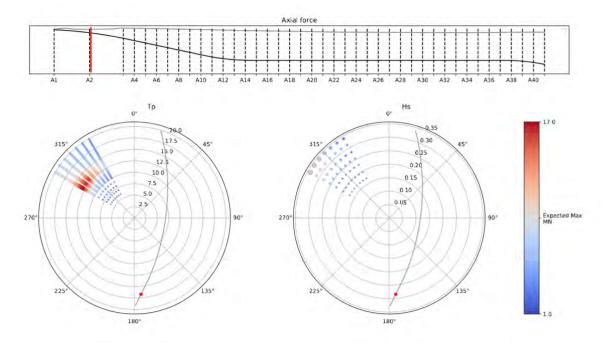
Figure 2-4: Axial force in the bridge girder at the tower for 100-year return period swell sea states.
