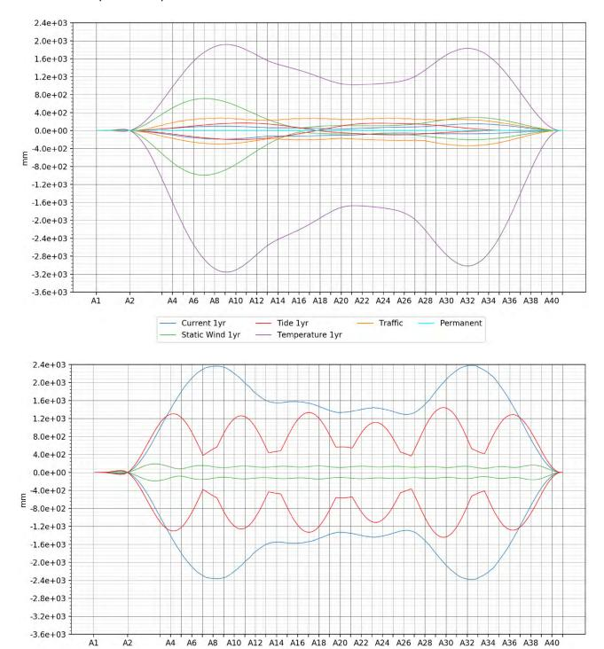
Figure 4-13 Overview of contributions to transverse displacements from slowly varying (top) and wave and wind (bottom) load components for the K12\_07 concept, 1 year return period.
