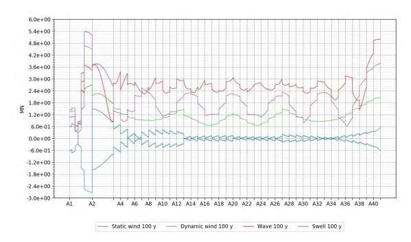
Figure 4-7 Overview of transverse shear force contribution from slowly varying loads (top) and wave and wind loading (bottom) for the K12\_07 concept.
