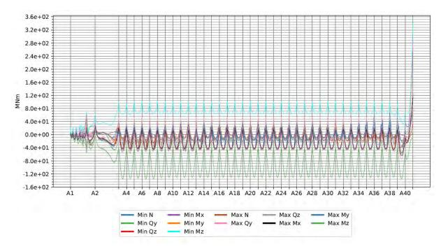
Figure 3-11 Traffic loads - Weak axis bending moment in bridge girder (envelope values) [MNm]
