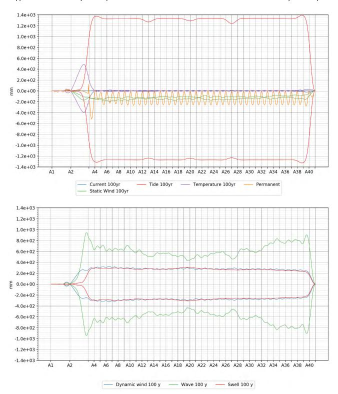
Figure 4-10 Overview of contributions to vertical displacements from slowly varying (top) and wave and wind (bottom) load components for the K12\_07 concept, 100 year return period.
