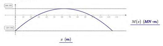
The stay cable forces in K12\_07 are verified by hand-calculations based on that each stay cable in front span have a vertical component corresponding to  $\frac{137.3+49.1}{2}\frac{kN}{m}\cdot 20m=1864kN$  plus half the cable weight. The back span stay cables are determined by horizontal equilibrium about the pylon. The results and comparison are presented below:
