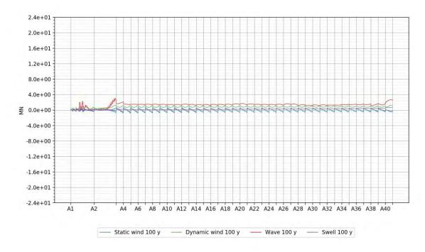
Figure 4-6 Overview of vertical shear force contribution from slowly varying loads (top) and wave and wind loading (bottom) for the K12\_07 concept.
