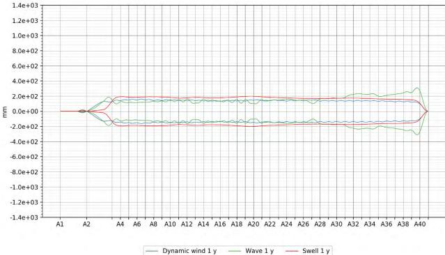
Figure 4-14 Overview of contributions to vertical displacements from slowly varying (top) and wave and wind (bottom) load components for the K12\_07 concept, 1 year return period.
