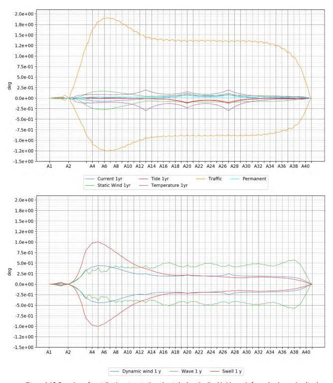
Figure 4-15 Overview of contributions to rotation about the longitudinal bridge axis from slowly varying (top) and wave and wind (bottom) load components for the K12\_07 concept, 1 year return period.
