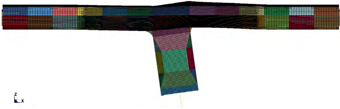
Figure 3-18 Model with shear force in x-direction, deformed model
