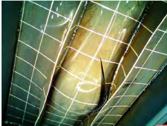
(a) Experimental failure mode, from Alsos (2008)
