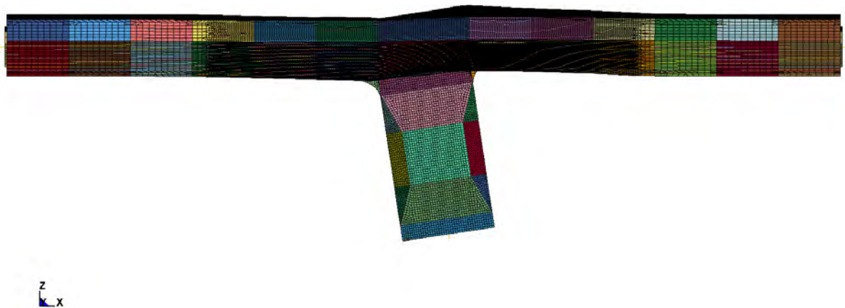
Figure 3-2 Model with shear force in x-direction, deformed model
