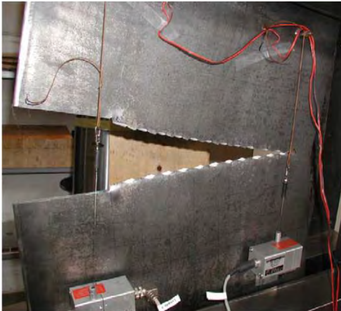
Figure A-6 Plate tearing test apparatus
