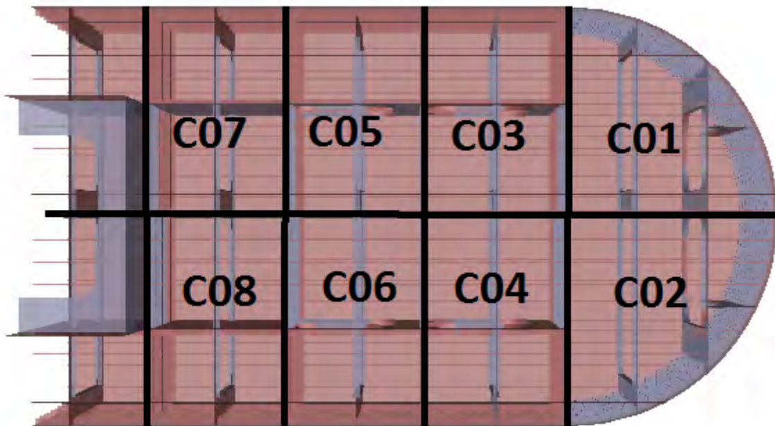
Figure 4-41 Compartment numbering in pontoon
