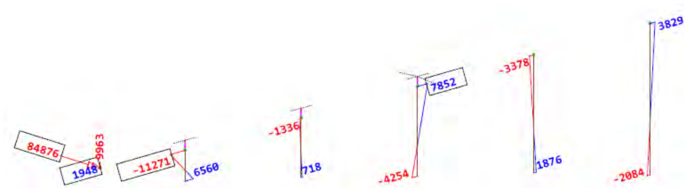
Figure 6-15 FSHB. Permanent loads. Side span piers and abutment. Bending moments [kNm]
