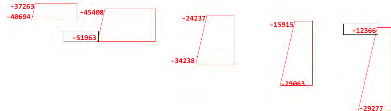
Figure 6-27 FSHB. Ship impact simulation. Side span piers. Axial force including permanent loads [kN]
