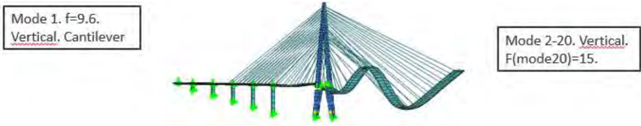
Figure 6-31 FSHB. Buckling modes and critical factors ( N_{cr}/N_{Ed} )
