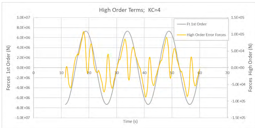
Figure 21 : 1st order Fitted Signal (grey) and High order signal (Orange, amplified scale): difference between 1 st order and CFD resultant forces. (different scale both signals)
