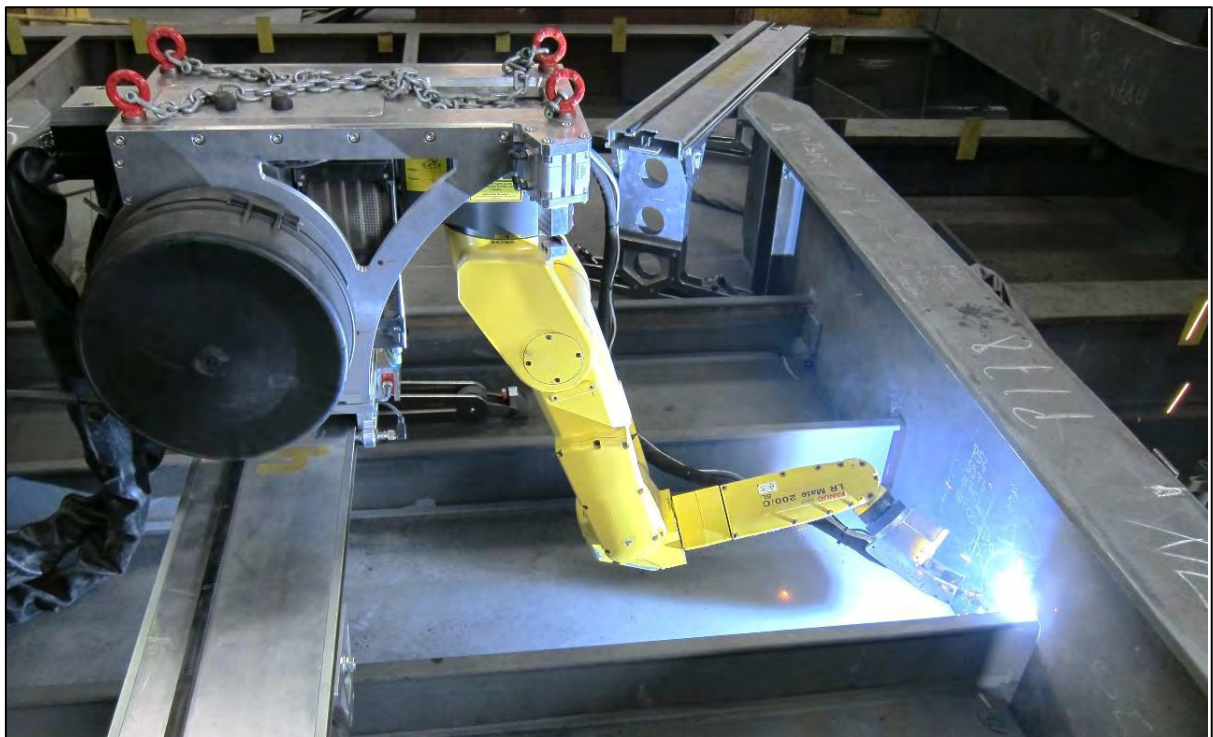
Figure 16-9 Robotic welding concept which might also be used for fillet welds between diaphragms/stiffeners, troughs and deck
