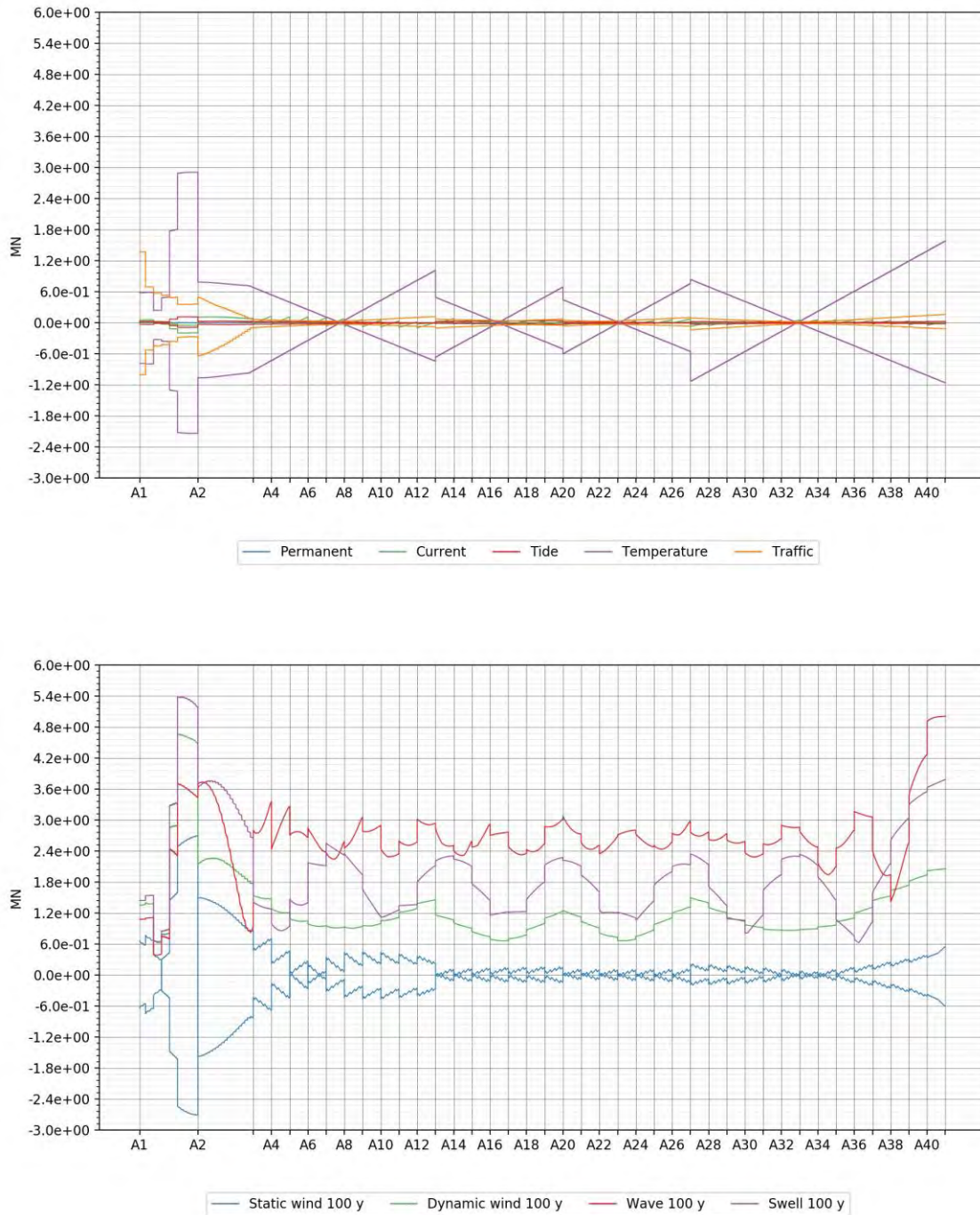
Figure 6-13 Overview of transverse shear force contribution from slowly varying loads (top) and wave and wind loading (bottom) for the K12_07 concept.
