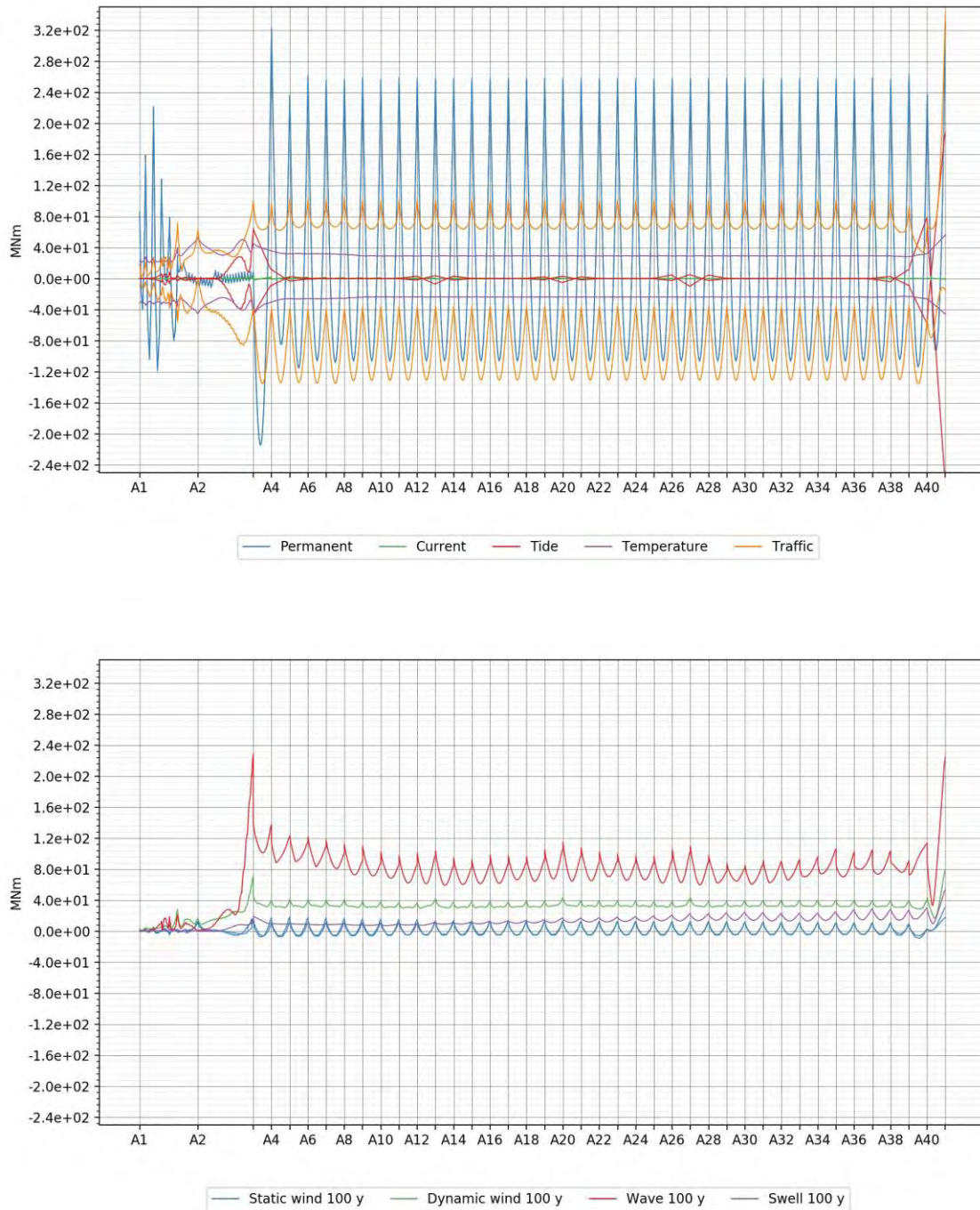
Figure 6-10 Overview of weak-axis bending moment contribution from slowly varying loads (top) and wave and wind loading (bottom) for the K12_07 concept.
