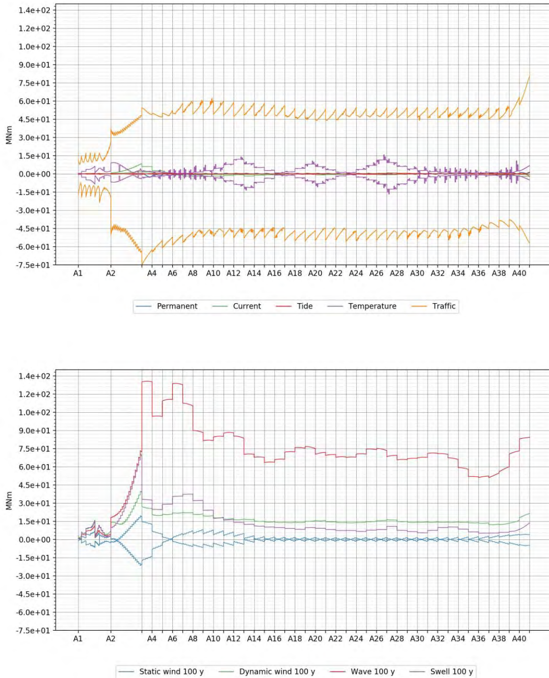
Figure 6-11 Overview of torsional moment contribution from slowly varying loads (top) and wave and wind loading (bottom) for the K12_07 concept.
