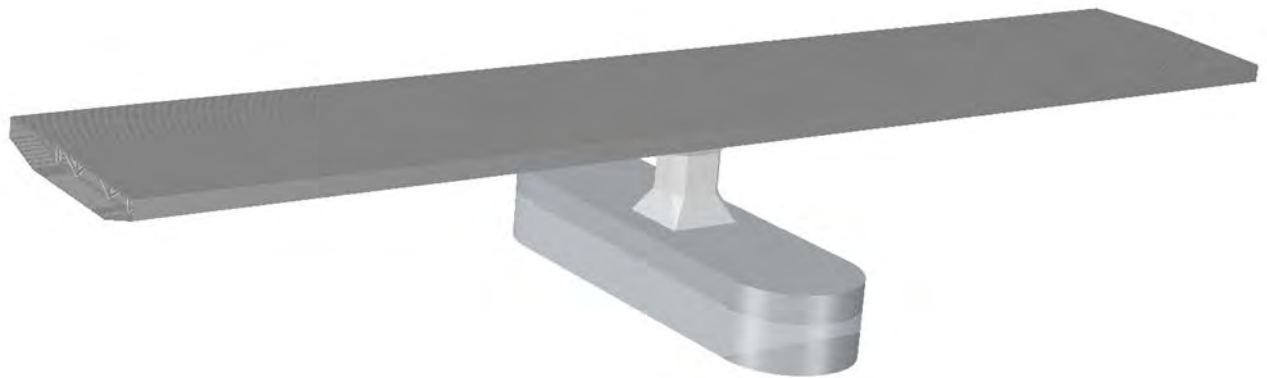
Figure 6-1 Typical floating bridge at lower part showing bridge girder, column and pontoon
