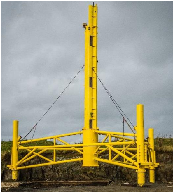
Figure 5-10. Drill rig MK2 /20/ with adjustable legs for levelling at the seabed
