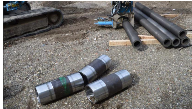
Figure 5-16. Carbide cross cut Ø340 mm, Titan 196/130, 3 m long, Coupling nut Ø254 x 600 mm.
