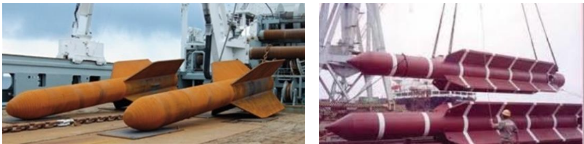
Figure 5-5 DPA (left) vs. torpedo pile concept (right). Source: www.deepseaanchors.com and www.offshore-mag.com .
