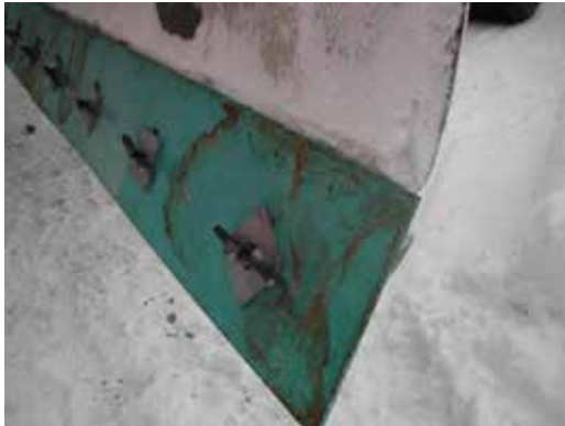
Figur 4-38 a) Slett vegstål - b) Perforert stål (P300)
