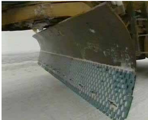
Figur 4-38 a) Slett vegstål - b) Perforert stål (P300)
