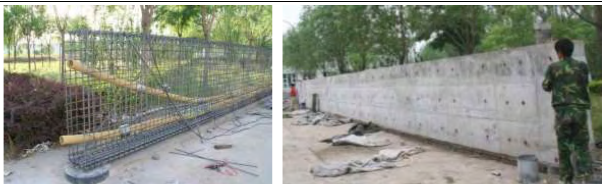
Figure 2 Large-scale experimental beam
