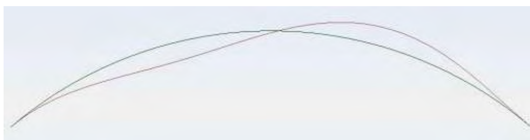
Figure 9 Buckling mode number 1 (in the horizontal plane)
