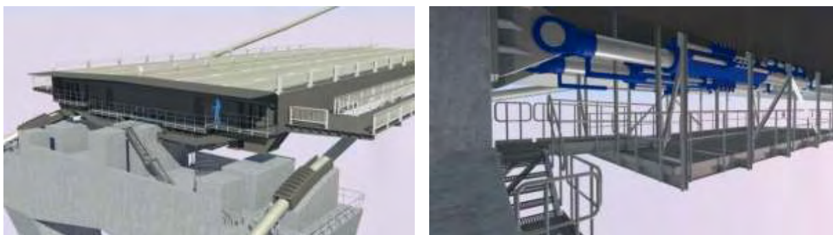
Figure 2: Deck end at side span pier, deviation saddles (left), hydraulic buffers connected to side span pier (right)
