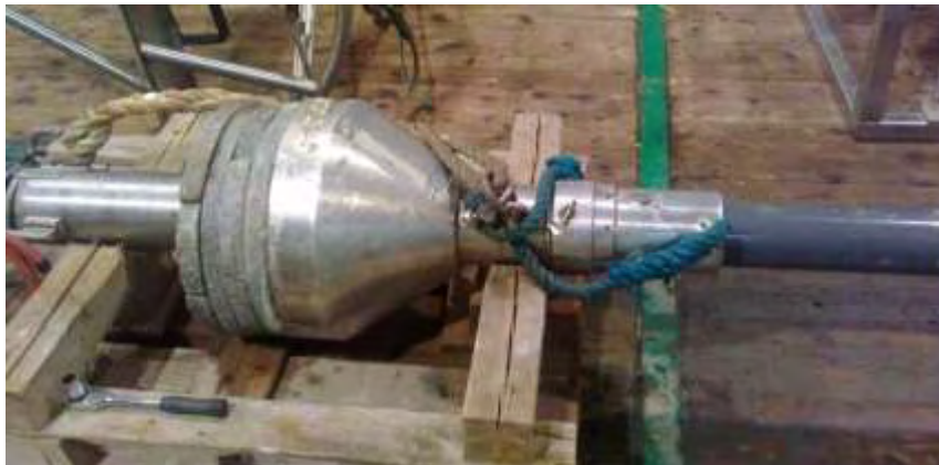
Figure 4: Gravity corer with adjustable weight
