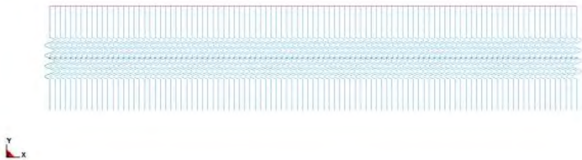
Fig. 9 Finite element analysis model(100 beam elements and 101 spring elements)
