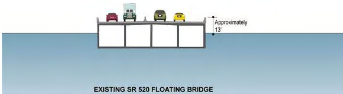
Figure 3 – Existing SR 520 Floating Bridge, 18.29 m wide (note 13 feet = 3.96 m)
