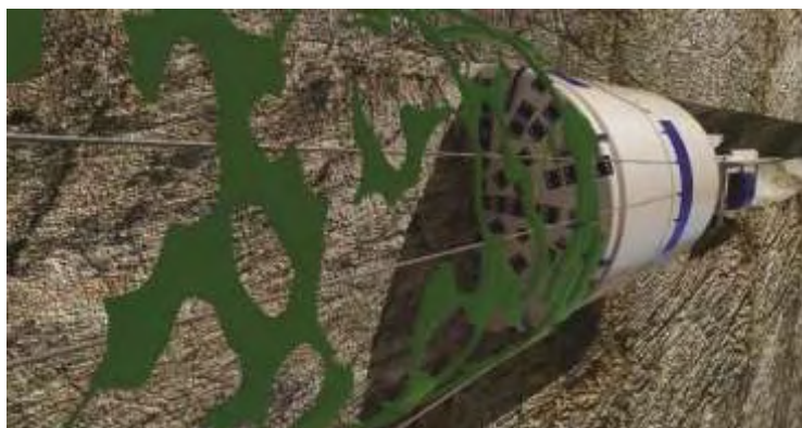
Figure 6. Double shielded Robbins TBM with the possibility of probing ahead of tunnel face and pregrouting
