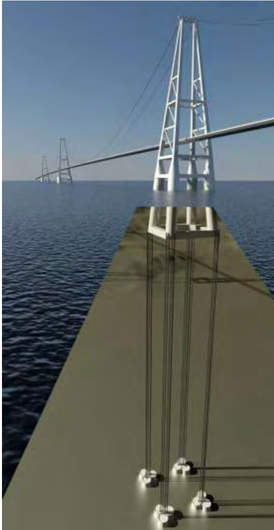
Fig. 6: Boknafjord Floating Foundation
