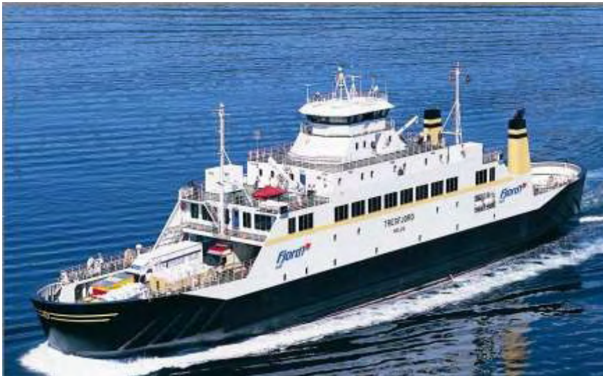
Fig. 9 "Tresfjord" converted from diesel electric to gas electric ferry
