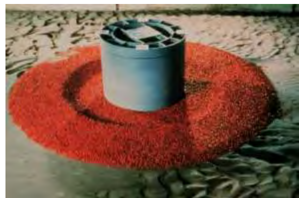
Photo 3 Scouring test with protection model
