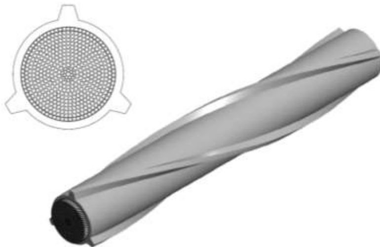
Figure 7: Cross-section and isometric view sheathed spiral strand with helical strakes.
