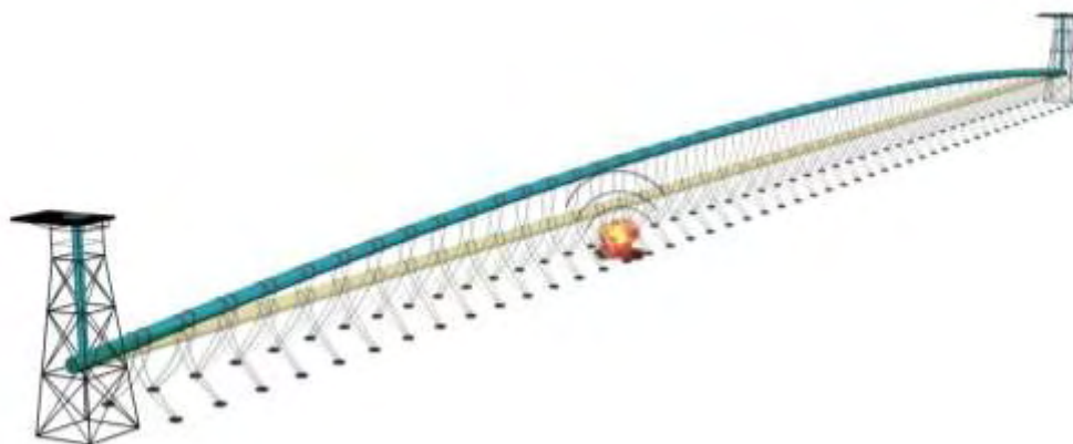
Fig. 4 The body of submerged floating railway attacked by underwater explosion
