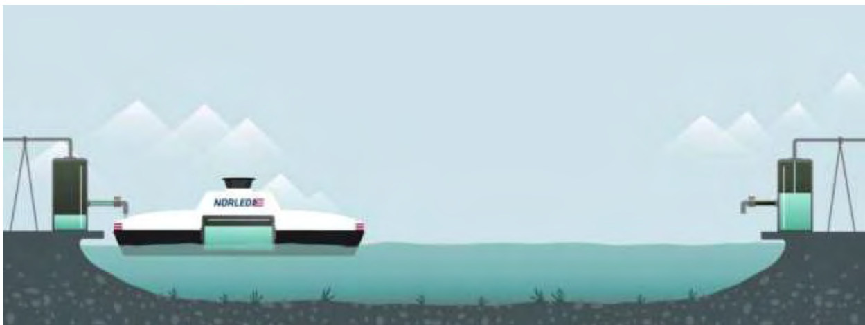
Fig.8 Illustration showing principle with a battery bank continuously charged from the public grid.
