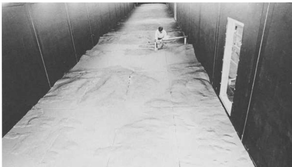
Figure 1: Topographical model of the Norwegian West Coast. View downwind from the North Sea (Davenport and King, 1990).
