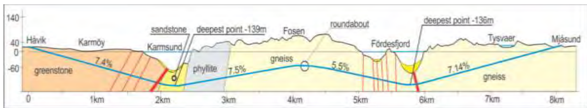
Figure 6. Longitudinal profile with geology of the T-connection subsea tunnels. Red lines indicate the main weakness zones encountered during tunnelling.
