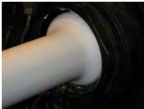
Figure 4: “Tube down” of the molten plastic.
