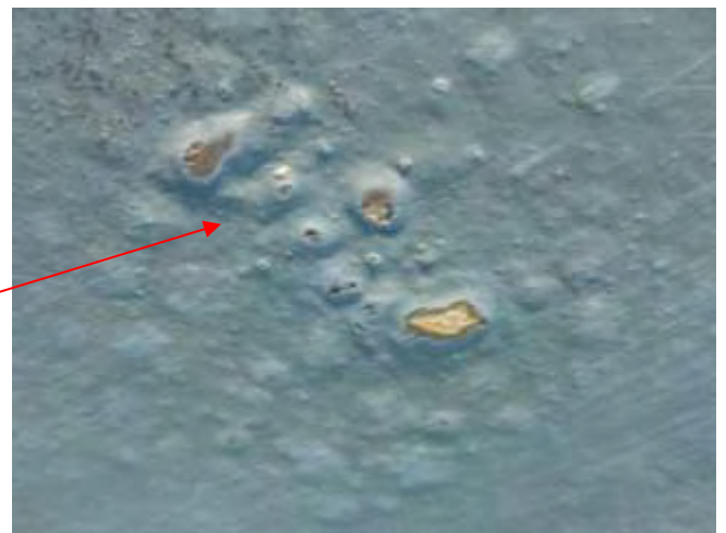
Photo no. 7 Penetration of corrosion products from TSZ through paint system (22 years)
