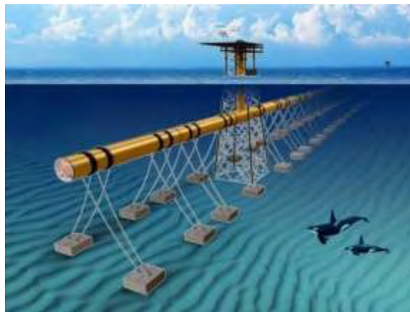
Fig. 2 Submerged floating railway shaped as pipe line
