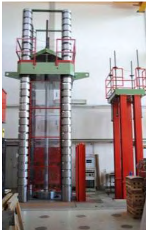
Figure 3: Left side: 30,000 kN testing machine; right side: 10,000 kN testing machine
