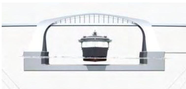
Figure 4 Light framework arch bridge
