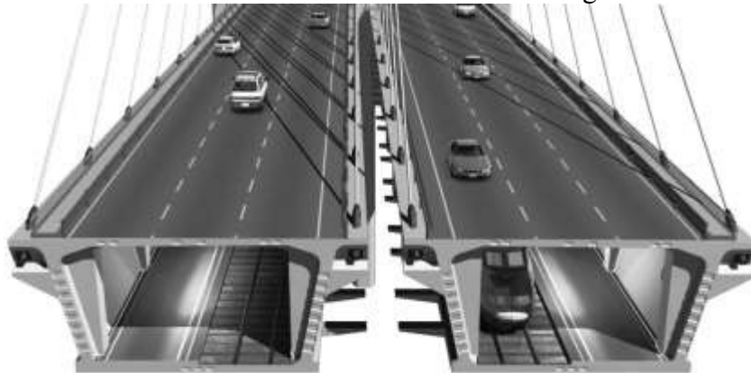
Fig.1 Twin Girder of the Saivan Bridge
