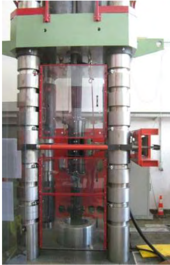
Figure 4: 30,000 kN testing machine with deviation device for dynamic bending deviation
