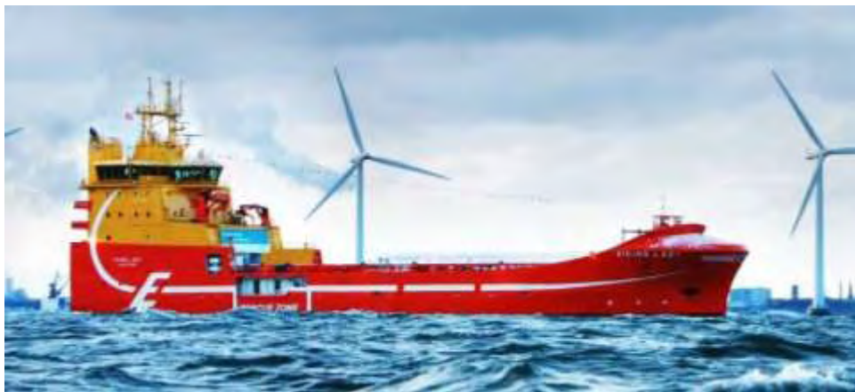
Figure 1. Eidesvik's Viking Lady is ready to install its 0.5 MWH battery system in March 2013.
