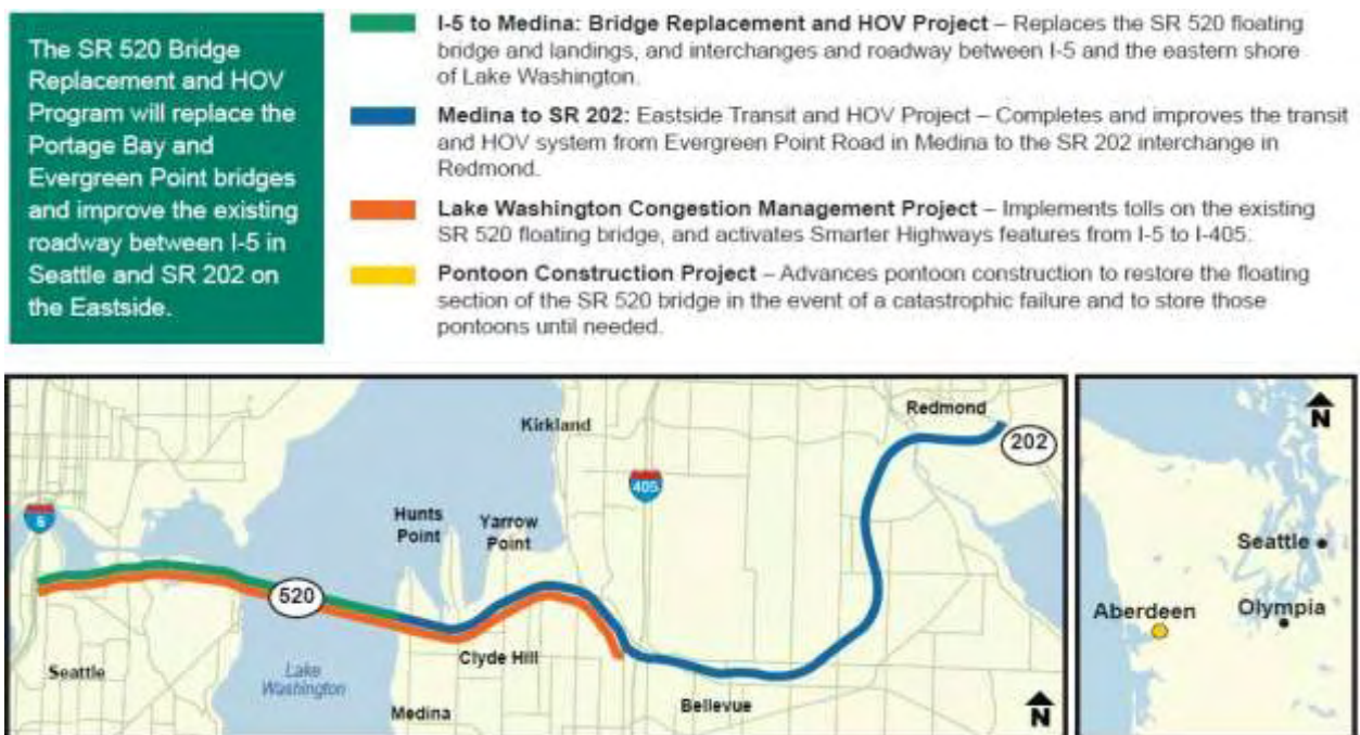
Figure 2 – SR 520 Replacement Program
