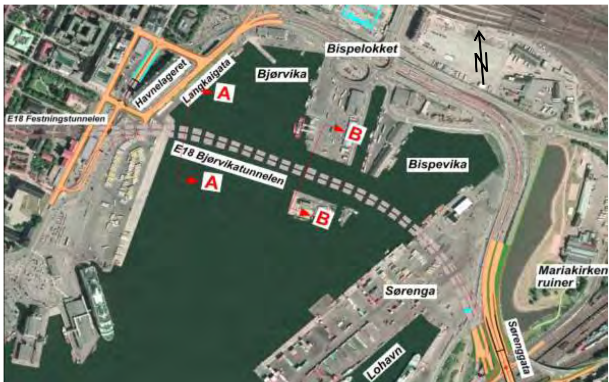
Figure 1- Plan view of the immersed tunnel across the Bjørvika bay in Oslo
