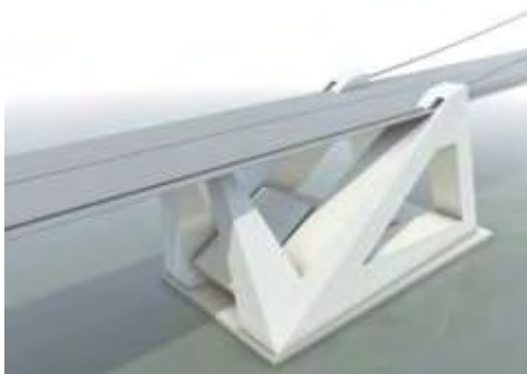
Figure 19: Concept for a seismically isolated anchorage
