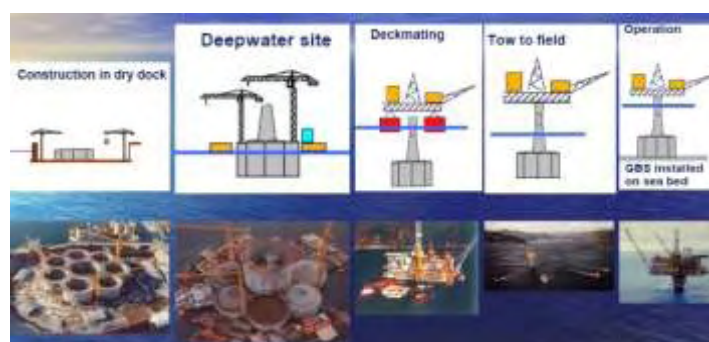
Fig.5. Construction of a gravity based concrete platform
