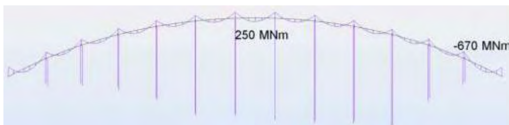
Figure 7 Horizontal bending moments for traffic loads
