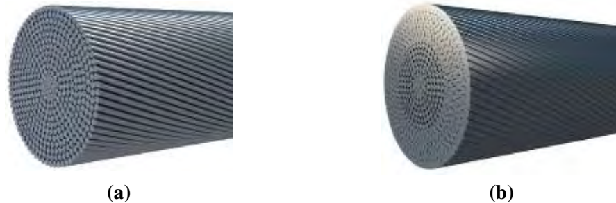
Figure 1: Rope constructions for structural applications, (a) Spiral strand, (b) Locked coil strand.
