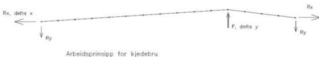
Figure 2. Static equilibrium of the chained bridge
