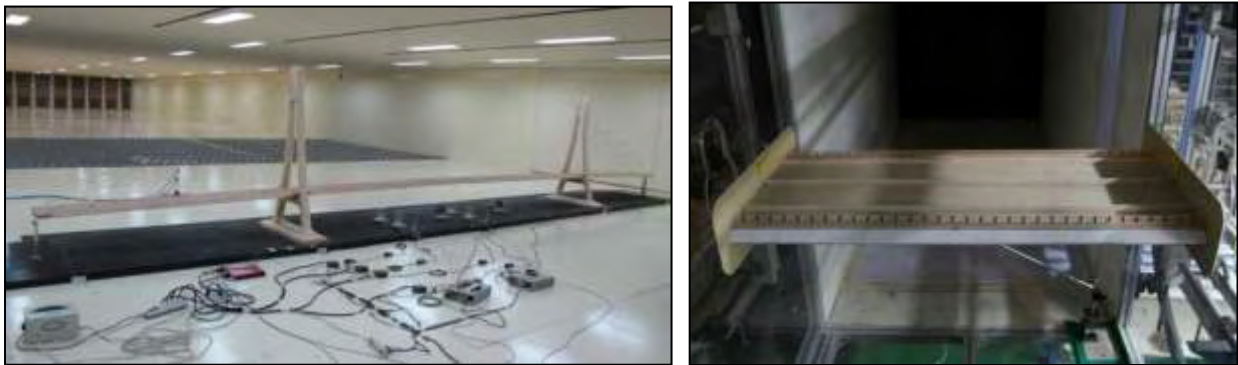
Figure 11: Global model and typical cross-section in wind tunnel test in Korea
