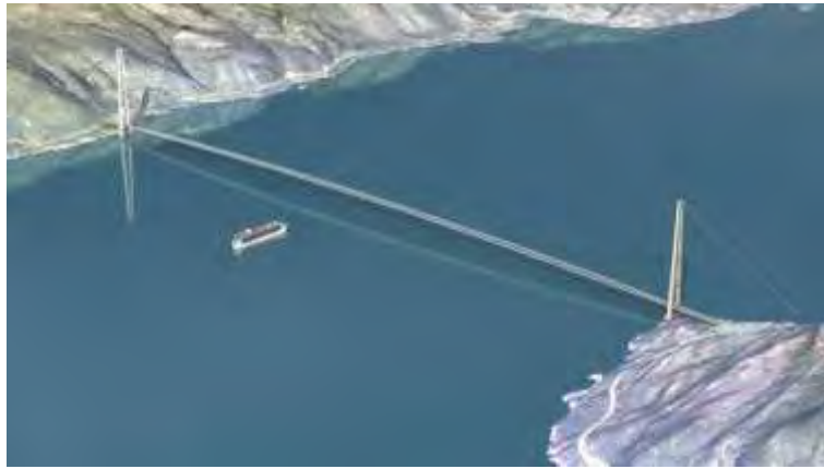
Figure 1 Suspension bridge with a main span of 3700 m (Ill: Norwegian Public Roads Administration)
