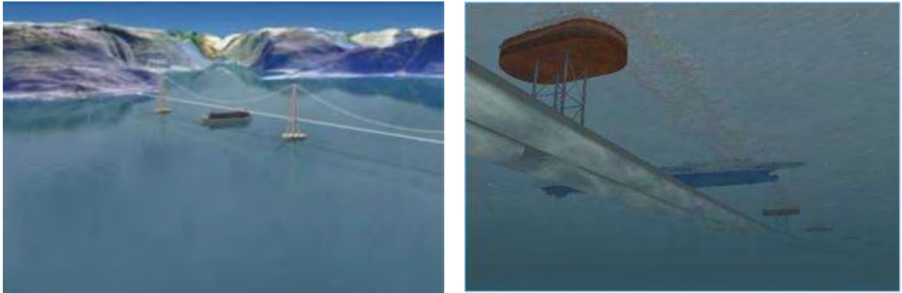
Figure 2. Conceptual bridge designs. Floating bridge (left) and submerged floating tunnel – SFT - (right).
