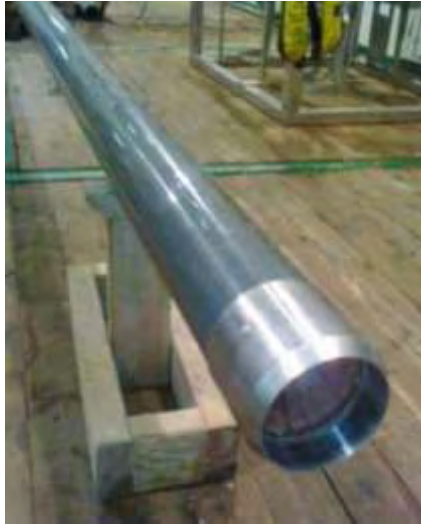
Figure 5: PVC-tube mounted with steel edge and sample protection
