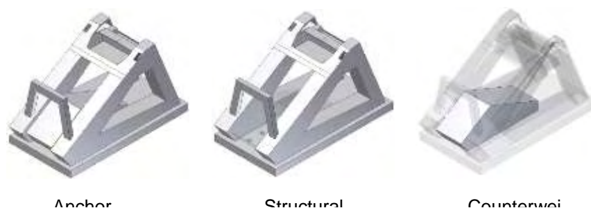
Figure 20: The anchorage is divided into a structural part and a non-structural isolated counterweight
