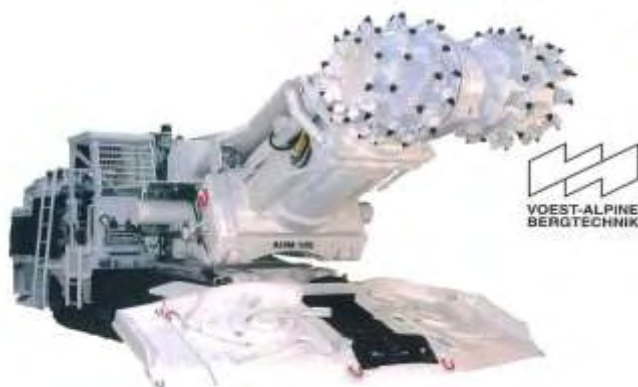
Figure 8. Roadheader for mechanical excavation (example: Voest Alpine).
