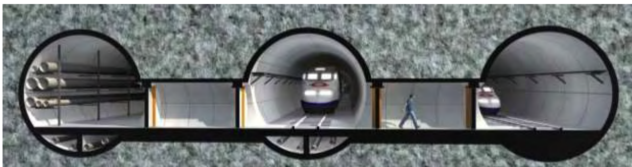
Figure 4. Option with 3 tunnels (outer diameters: 6.6 m).
