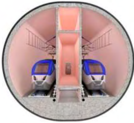
Fig. 2 Section of submerged floating railway
