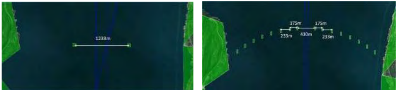
Figure 3. Pontoon distances. Floating bridge (left) and SFT (right).
