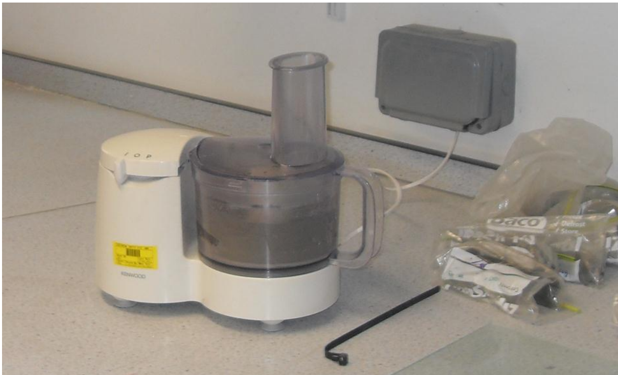
Figure 4-1 Mini food mixer used to mix the dry sample with distilled water
