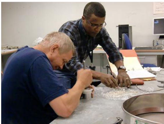
Figure 5-1 Sample preparation for the modified falling cone test method
