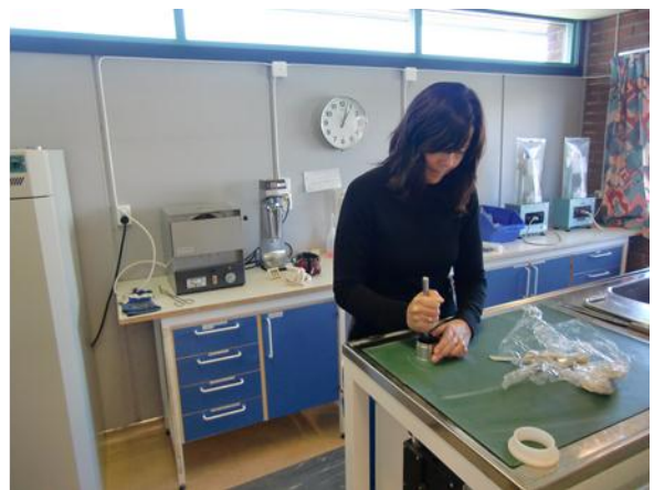
Figure 5-1 Sample preparation for the modified falling cone test method
