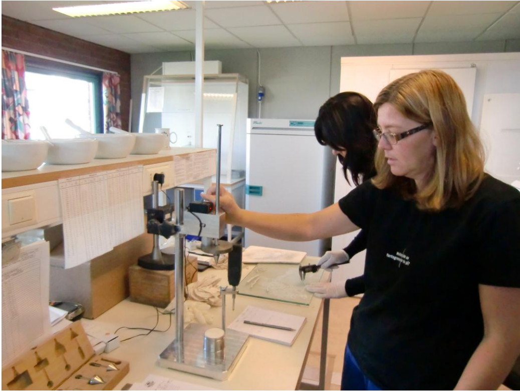
Figure 5-2 Parallel tests to determine the w_p of Speswhite kaolin using the proposed falling cone and standard method
