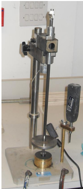
Figure 3-3 Proposed plastic limit measuring device
