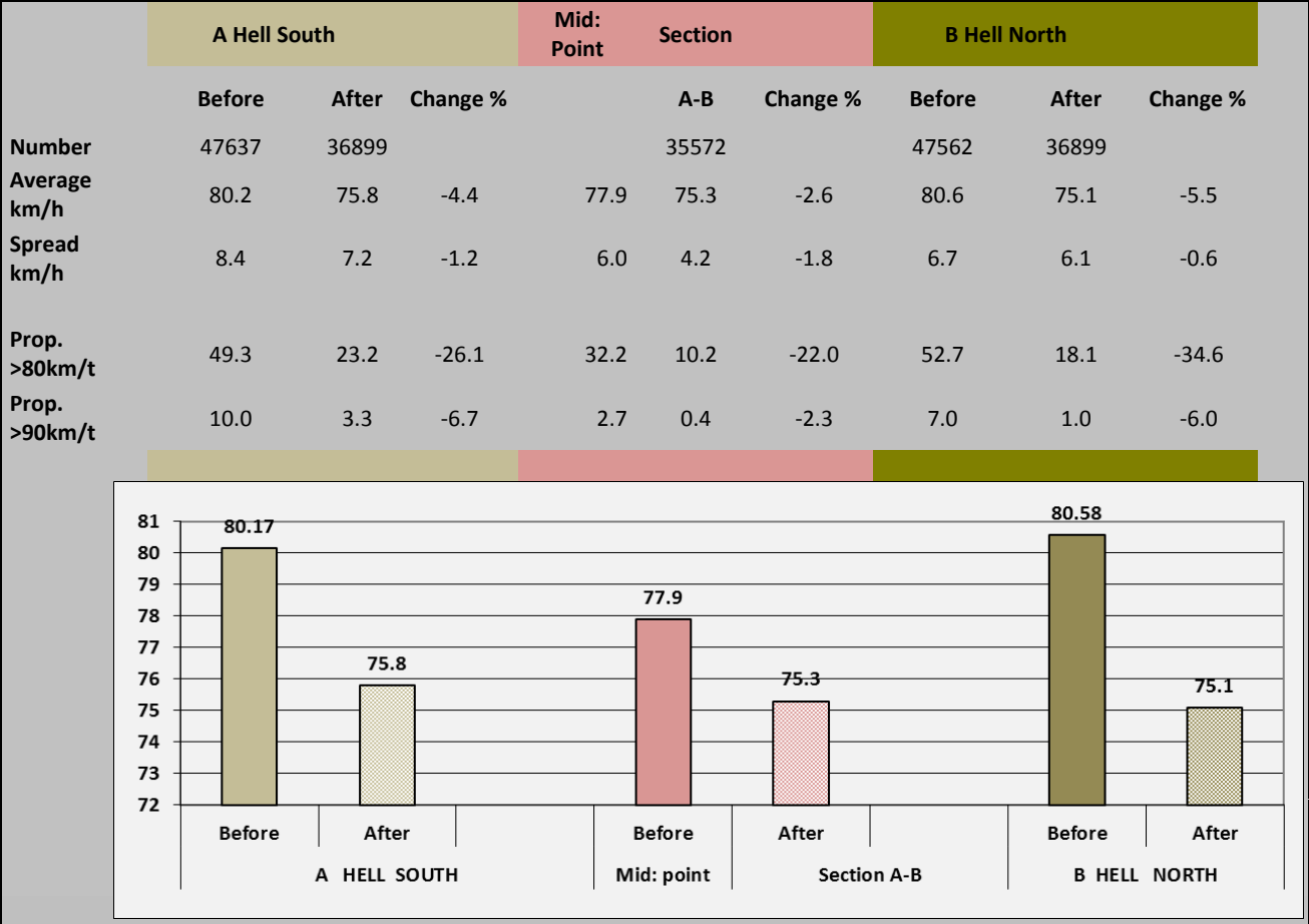
Figure 8: Before and after ASSC, Hell tunnel, E6, Trøndelag. No. of vehicles, average speed, spread and percentage over 80 and 90 km/h. At camera in point A (south Hell), on the section AB and at cameras in point B (north Hell).
