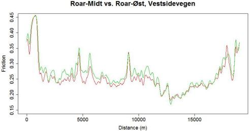
Figure 4: Comparing the estimated friction from RoAR-Midt (red) and RoAR-Øst (green).
