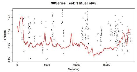
Figure 5: Comparing measurements from RoAR (red) with friction estimates from the two XC90 Volvo cars with quality higher than or equal to 5.
