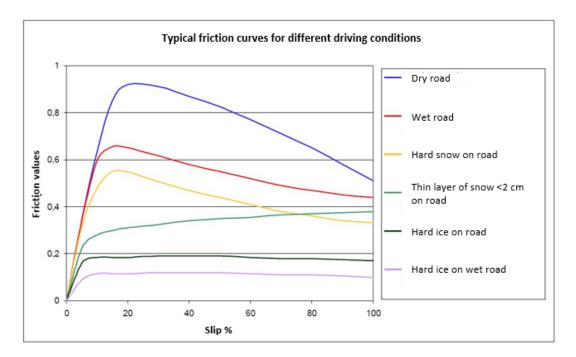
Figure 1: Typical friction curves for different road conditions. (Statens vegvesen & Norsemeter, januar. 1995)
