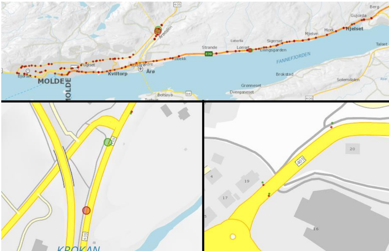
Figure 11 Signs detected in the Molde demonstrator. Point colors represent their source (red points are signs from NVDB, while green points are signs detected using the Vionice system). Point size represents the distance from the Vionice detection to the matching sign from NVDB.
