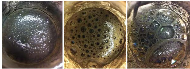
Figure 4.2: Typical foam structures, from left: fly ash 3, fly ash 2, fly ash 1
