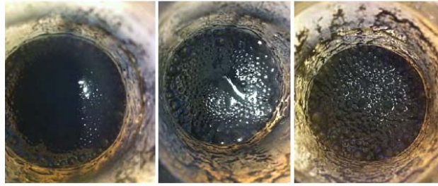
Figure 4.1: Foam propagation for high carbon ash, from left: initiation, filled surface, stable foam
