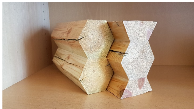
Figure 1 Model of the two elements making an oblique interlocked laminated timber deck
