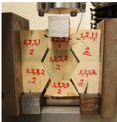
Figure 4 Shear testing in the laboratory with results /1/. Theoretical capacity due to rolling shear was calculated to 7.2 kN, about a third of the results.
