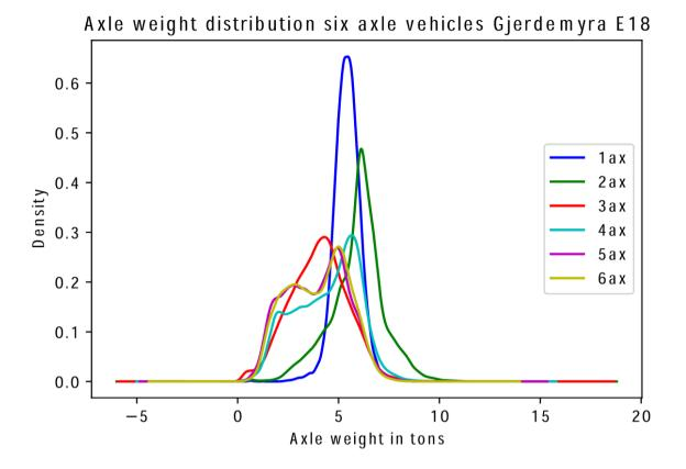
Figure 12 KDE plot raw axle weight data 6 axle vehicles Gjerdemyra E18
