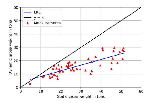
Figure 28 Static / raw and calibrated dynamic gross weights Losna E6
