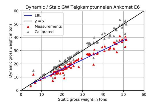
Figure 22 Static / raw and calibrated dynamic gross weights Teigkamptunnelen E6
