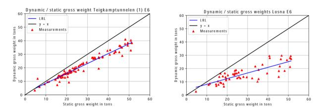
Figure 6 Field test results for ATK points Teigkamptunnelen and Losna along E6 in Oppland 2016
