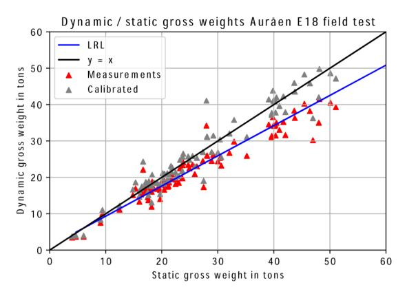
Figure 26 Static / raw and calibrated dynamic gross weights Auråen E18
