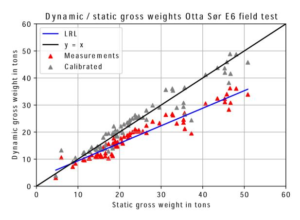
Figure 18 Static / raw and calibrated dynamic gross weights Otta E6
