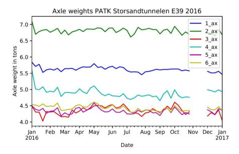
Figure 9 ATK data stability over time for all axels six axle semi-trailer vehicles at ATK Storsandtunnelen
