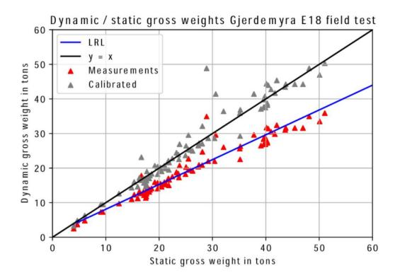
Figure 13 Static / raw and calibrated dynamic gross weights Gjerdemyra E18
