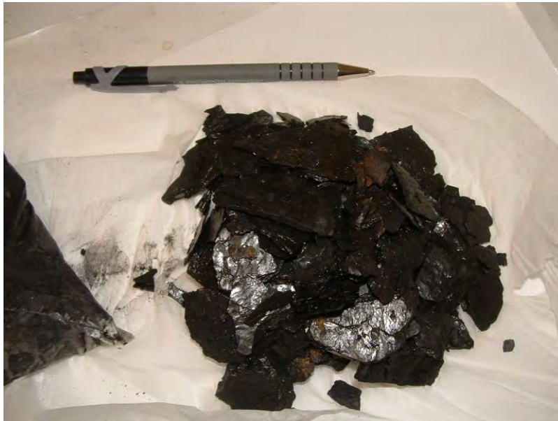
Figure A4-5-2: Svartdal tunnel Alum Shale core sample 320-06U after first manual crushing, representing a pure Black Shale without secondary calcite vein material.
