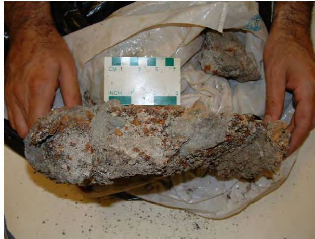
Figure 4: Spall V5, with extremely friable cement paste matrix from underneath layered Mn and Fe biofilm. Five year's old sprayed concrete from Locality 2c, Oslofjord subsea tunnel.
