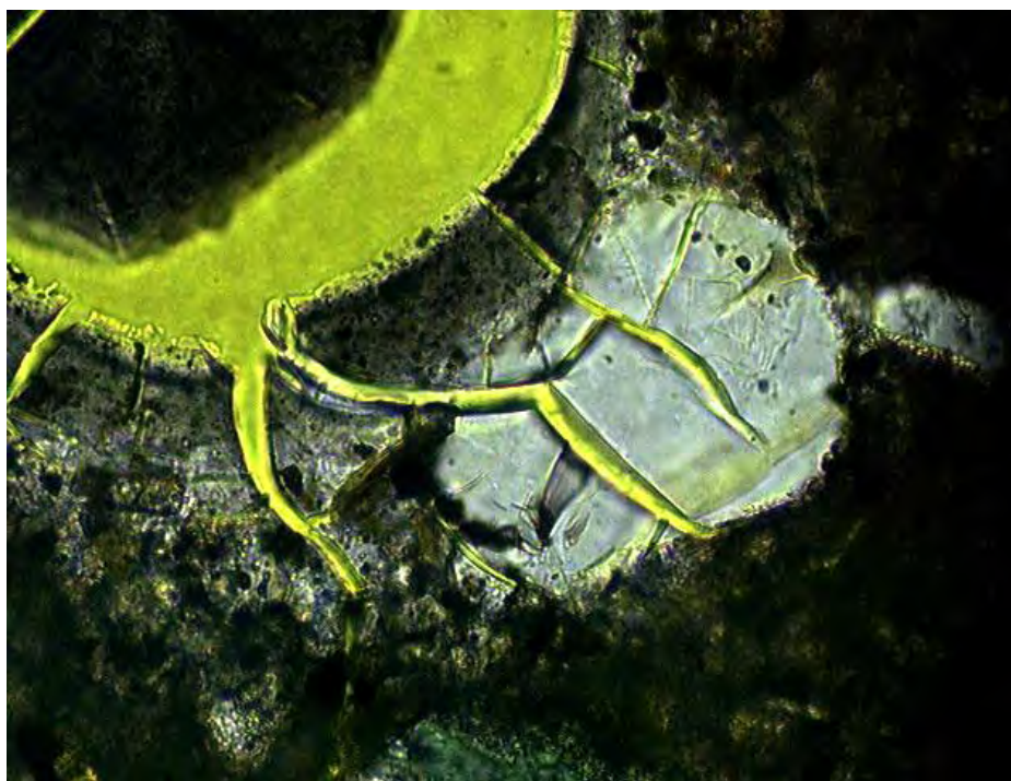
Figure A6-6-2 Detail of previous image showing SF with ASR-gel (light grey) which had formed at the margin against sound cement paste. Later desiccation cracks within SF and ASR gels. Note the absence of microcracks in the surrounding sound cement paste. Crossed polars (Width of field 150 \mu\text{m} ).
