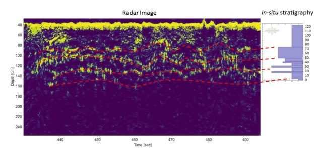
Figure 3: Left panel: Radar image showing intensity variations in backscattered energy (yellow means more energy) through snow depth (y-axis) and time (=distance on the x-axis). Right panel: In-situ stratigraphy from a snowpit dug in the transect. Blue columns show hand hardness of the different snow layers (horizontally elongated column indicates hard snow). The red dashed lines indicate our interpretation of the radar image.
