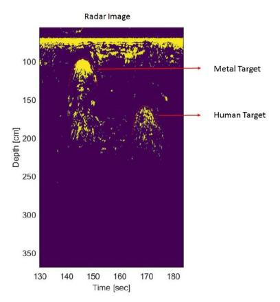
FIGURE 13 Post-processed GPR Image Showing Buried Objects at Site 1 (illustration: NORUT)
