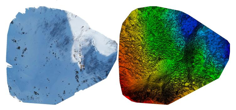
Figure 4. Orthomosaic and corresponding sparse Digital Surface Model before densification
