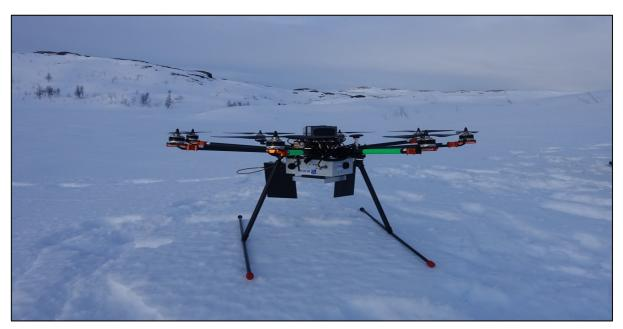
*Figure 1: UAV-borne radar system. The UWiBaSS is the grey box mounted beneath the UAV, with the transmitting antenna (grey plate) and both receiving antennas (black sheets) visible.*
