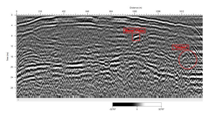
Figure 6. Metal plate and a person under the snow marked in the data
