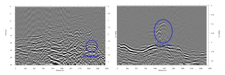
Figure 8.Car under the snow (left) and car parked on the road (right) data reflection patterns
