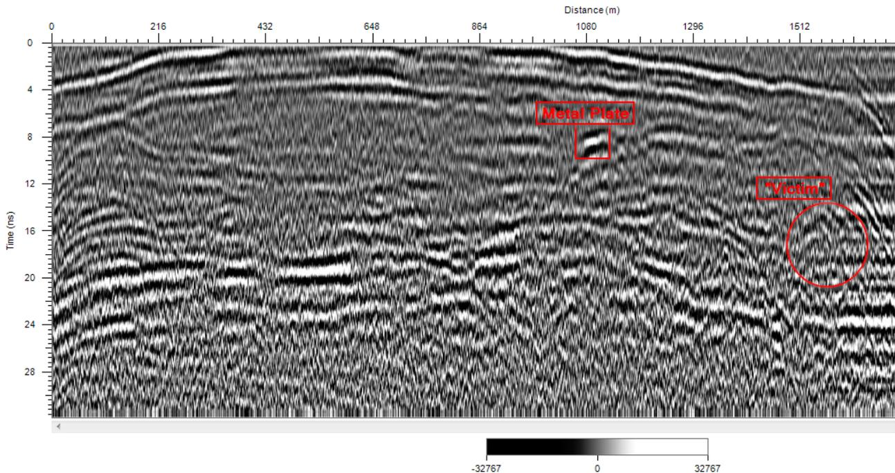
**Figure 6. Metal plate and a person under the snow marked in the data**
