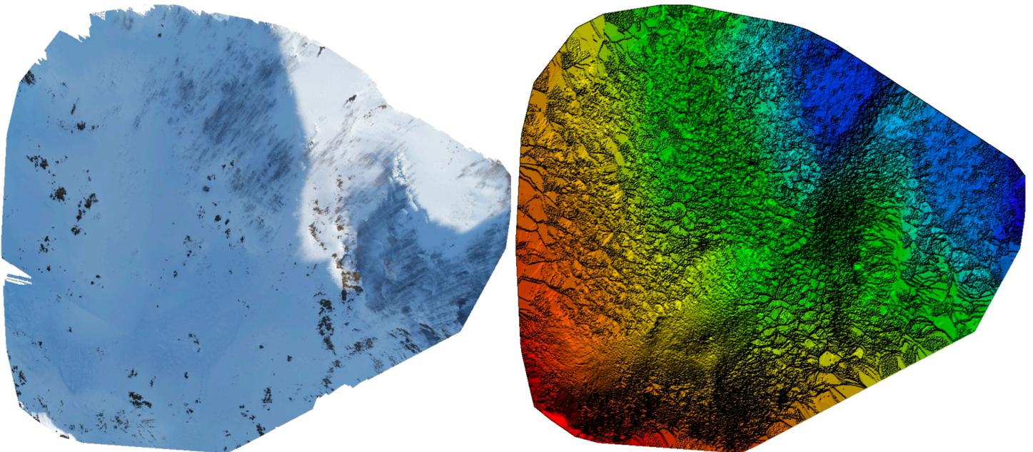
**Figure 4. Orthomosaic and corresponding sparse Digital Surface Model before densification**
