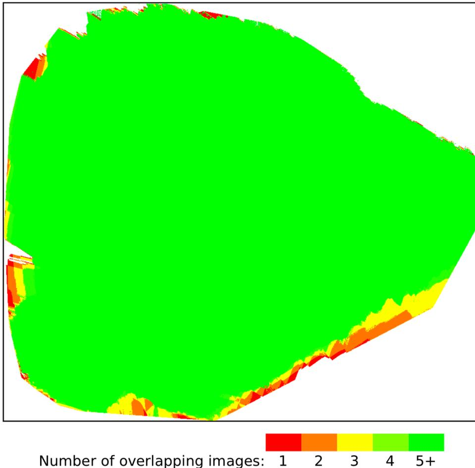
**Figure 2. Number of overlapping images computed for each pixel of the orthomosaic**
