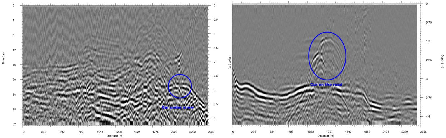
**Figure 8. Car under the snow (left) and car parked on the road (right) data reflection patterns**
