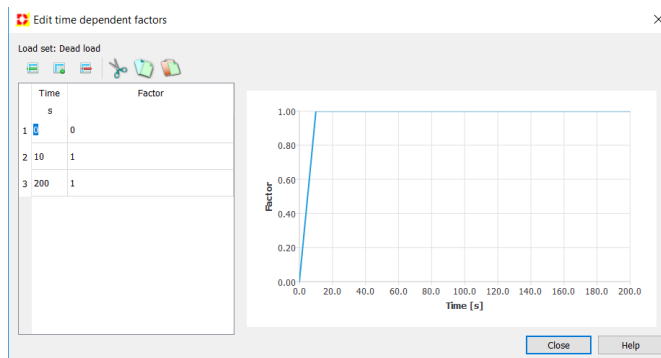
Figure 9.8: DIANA 2D model: Dead load; time dependent factor
