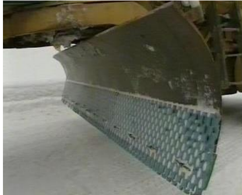
Figur 4-39 a) Slett vegstål b) Perforert stål (P300)
