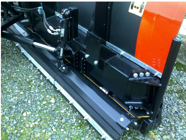
Figur 4-29 Hydraulisk betjente slapseelementer (Foto: Arctic Machine)
