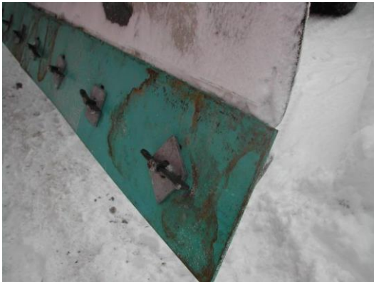
Figur 4-39 a) Slett vegstål b) Perforert stål (P300)
