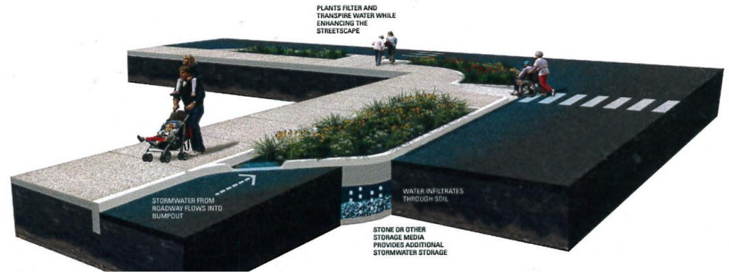
Corner Stormwater Bump-out
