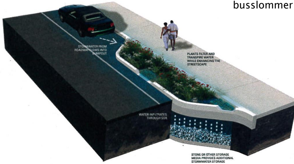
Mid-block Stormwater Bump-out
