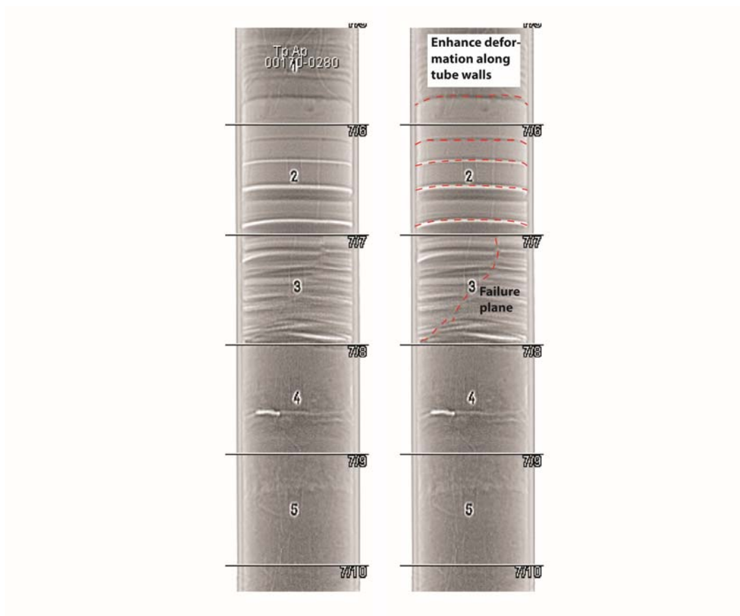
Figure 20: Example of x-ray imagery prior to extrusion for gross sample quality evaluation in a layered clay from Finneidfjord. The imagery shows enhanced deformation of layers along the cylinder walls and a failure plane in the loose sandy layers in the mid-section of the sample.
