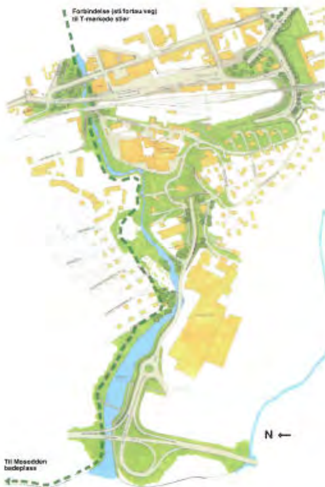
When the Mesnadal arm from the E 6 into the centre of Lillehammer was being planned and built, efforts were made to maintain a continuous green strip along the River Mesna. This starts at the T-marked paths on Stampesletta and ends at the bathing beach at Mosodden on Lake Mjøsa. The construction of a tunnel saved this beach from being destroyed by the E 6. Sources: Oppland Road Works Office and Knut Selberg Arkitektkontor
