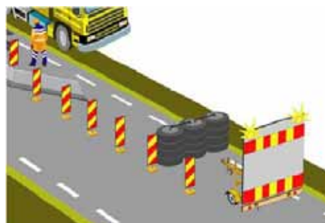
Figure 4.10 Protection equipment placed across the carriageway, with warning equipment.
