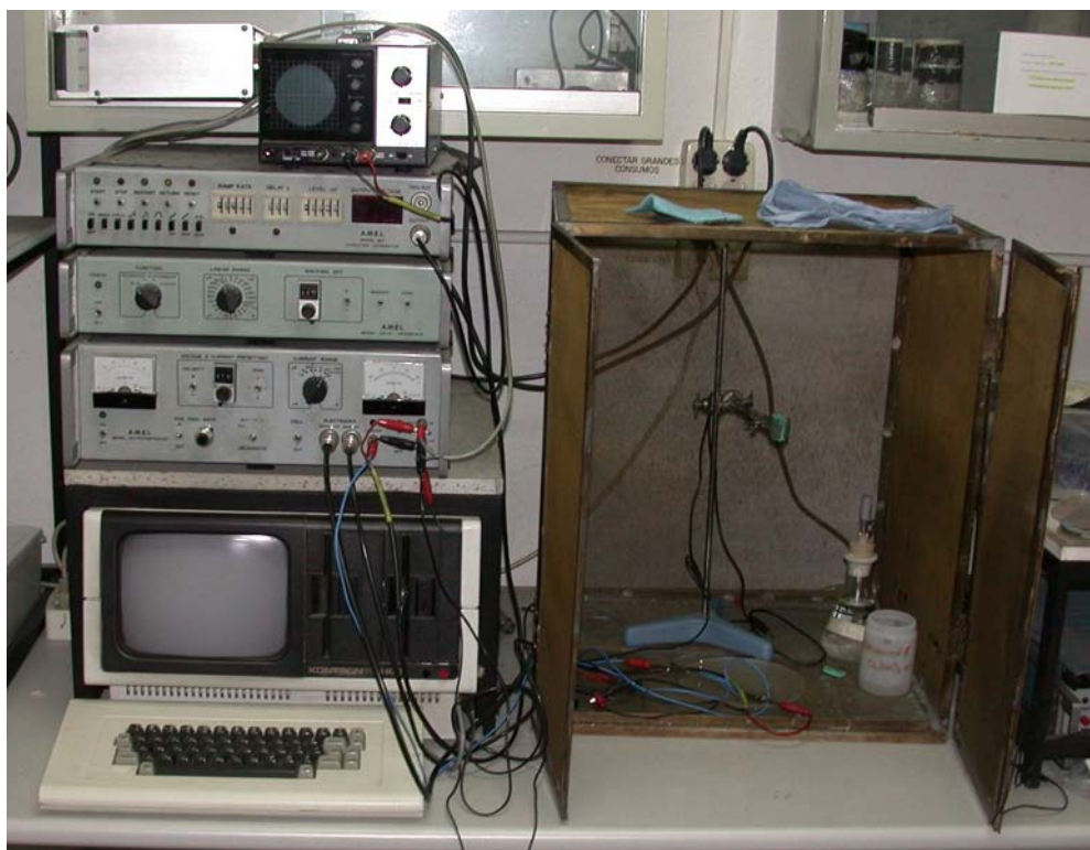
Figure 3. 11 Picture of the setup used for ohmic drop measurements
