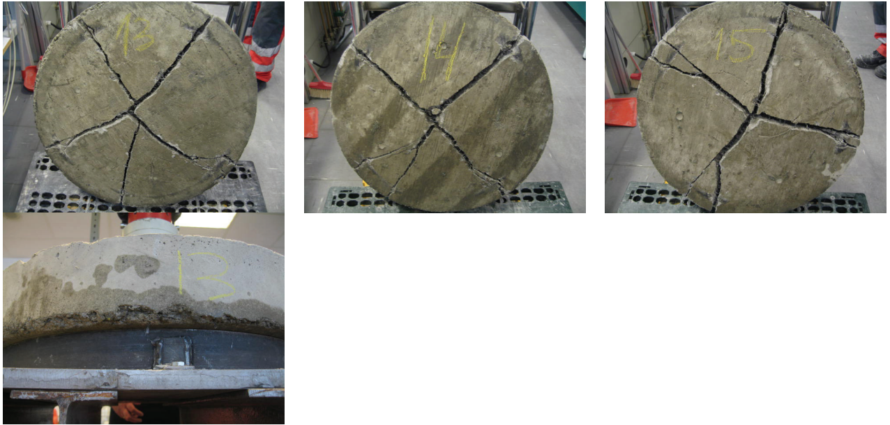
Fig. 7.6 Crack pattern, S9-7-BK-S (7 kg BarChip Kyodo, Sprayed, no bedding)
