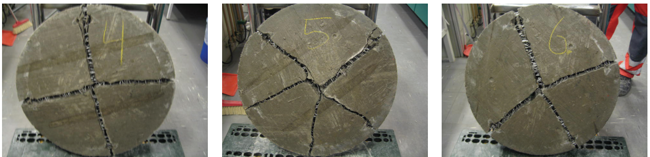
Fig. 6.2 Crack pattern, set S8-6-BC54-S (6 kg BC54, sprayed, no bedding)
