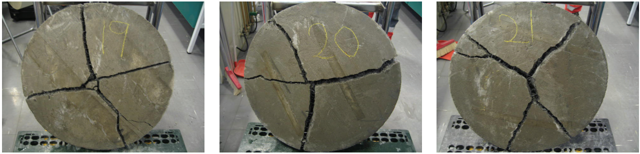
Fig. 6.7 Crack pattern, set S8-7-BK-S-PVC (7 kg BK, sprayed, PVC-bedding)
