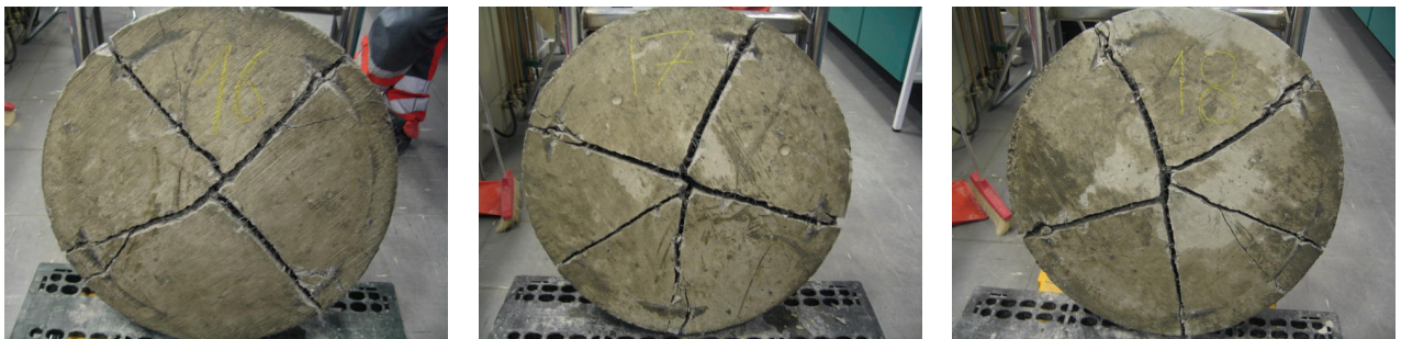
Fig. 7.7 Crack pattern, S9-8-BK-S (8 kg BarChip Kyodo, Sprayed, no bedding)
