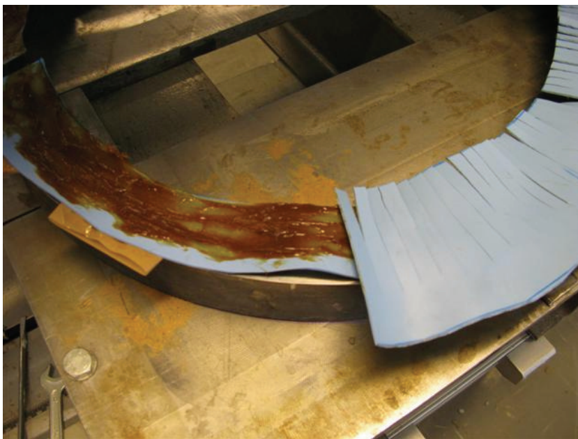
Fig. 5.4 Steel support with bedding of two layers of PVC with grease in between
