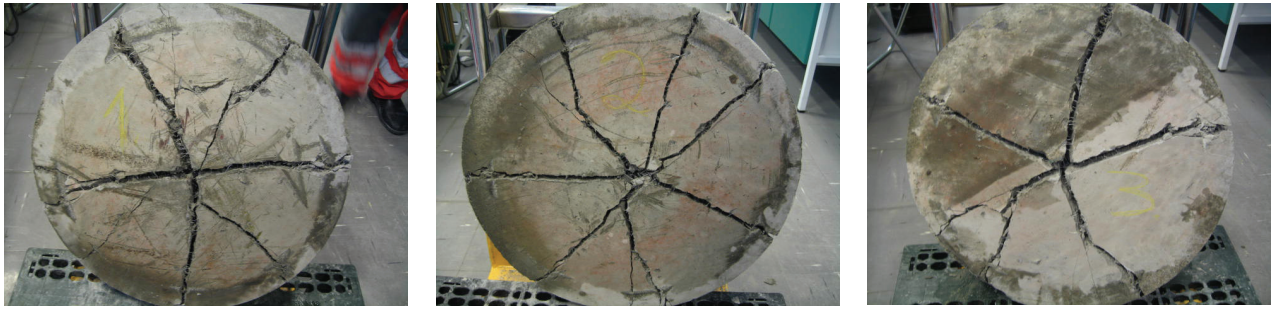
Fig. 7.2 Crack pattern, S9-20-D-S (20 kg Dramix, Sprayed, no bedding)
