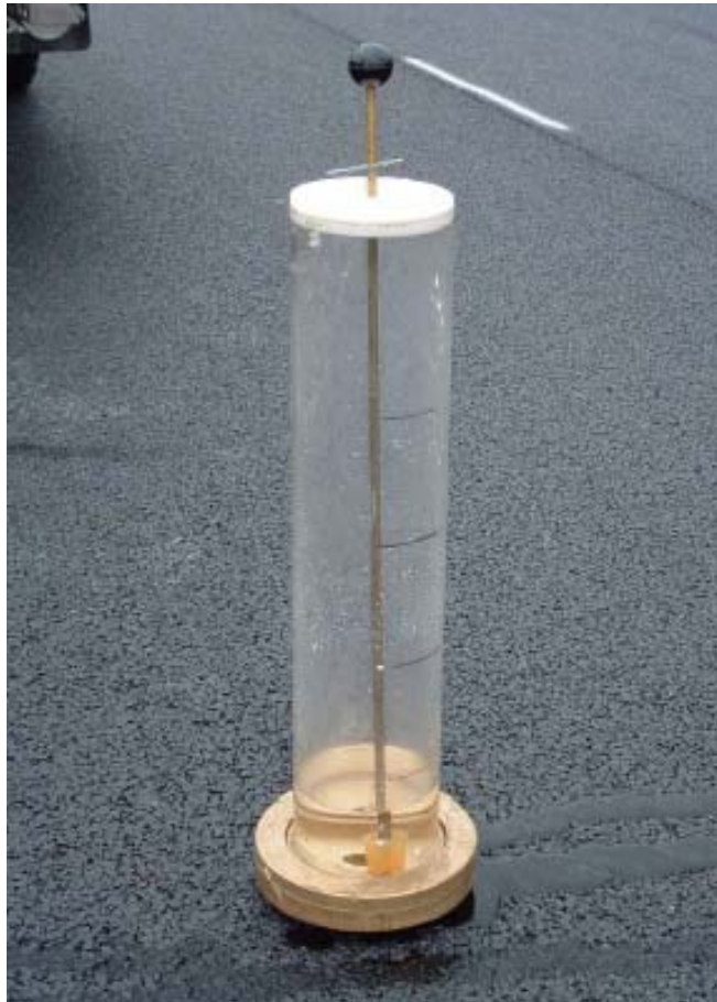
Figure 5 Equipment for permeability measurements (ref 18)
