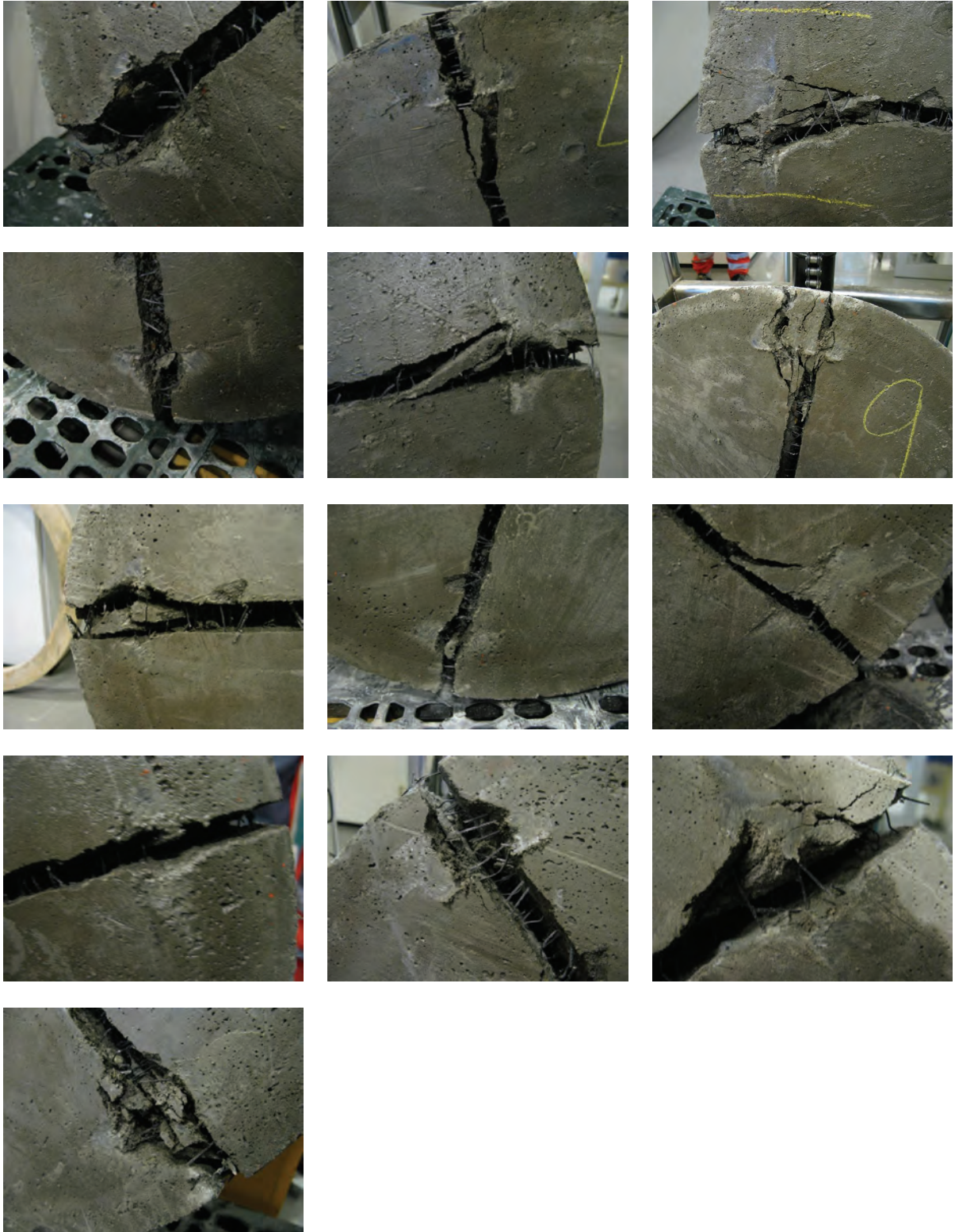
Close-up of crack-zones, Set 3: Steel support, no bedding
