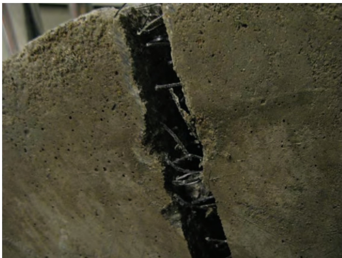
Fig. 7.9 Set 5: Steel support, two layers of Teflon as bedding material
