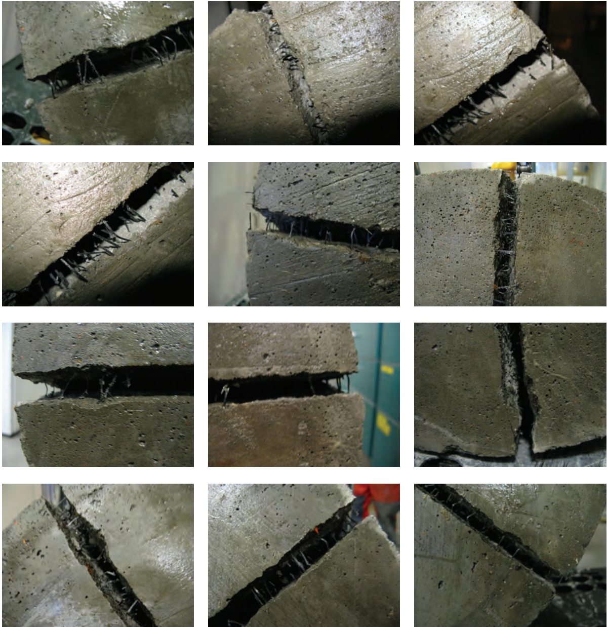
Close-up of crack-zones, Set 2: Steel support, two layers of PVC-membrane + grease as bedding material.
