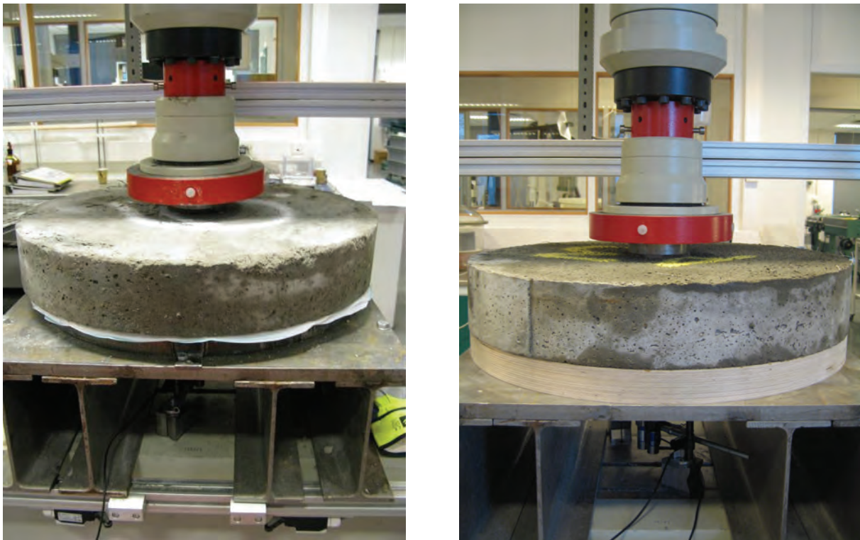
Fig. 5.1 Set-up for the energy absorption tests. Left: modified steel support (with Teflon bedding). Right: wooden support.
