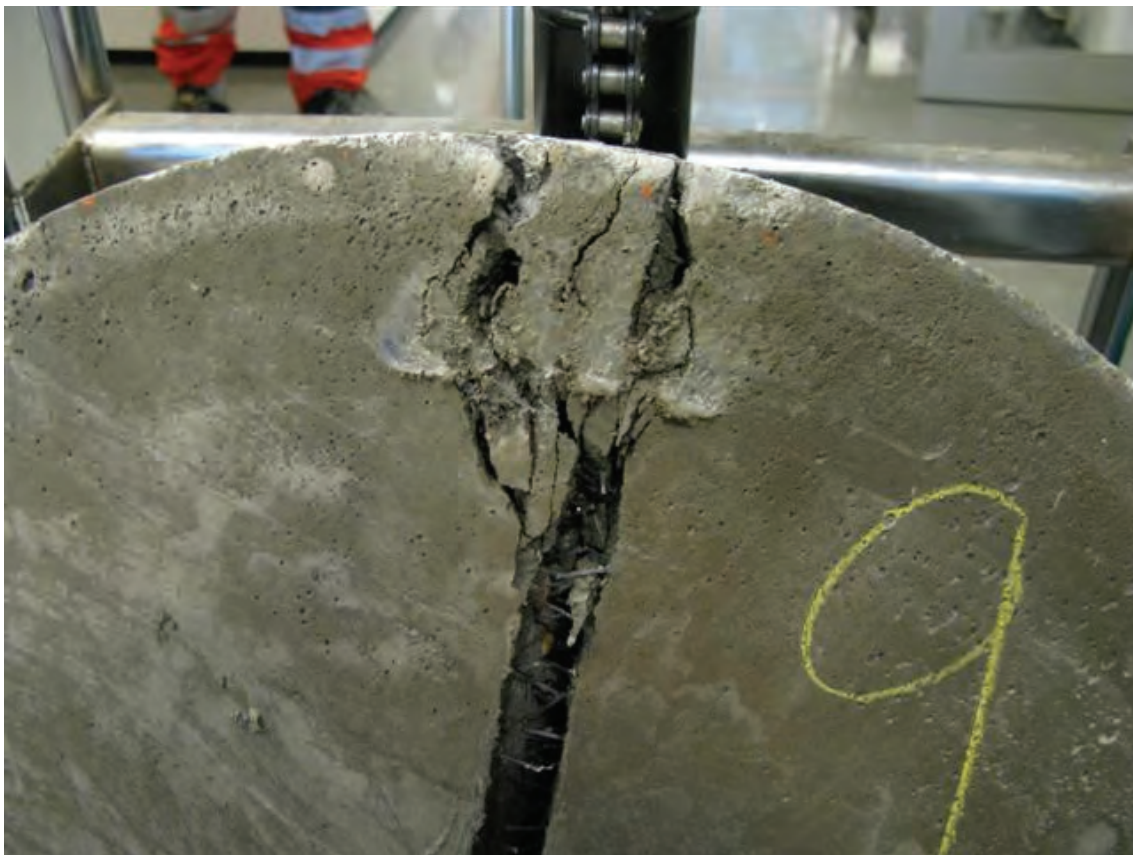
Fig. 7.7 Set 3: Steel support, no bedding
