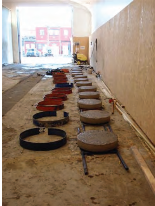
Fig. 4.3 De-moulding after 1.5 days.
