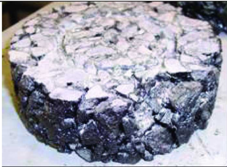
Figur 25: Da11 prøve kappet i to
