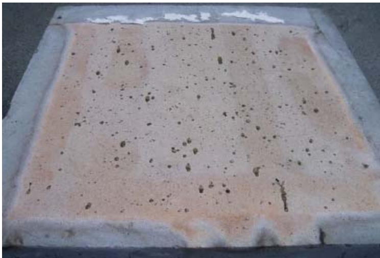
Figur 7 Lettbetong (skumglass) m/PP fiber eksponert for brann
