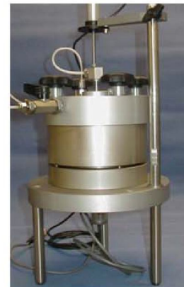
Fig. 4 GDS Rowe and Barden consolidation cell
