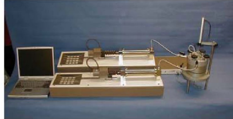
Fig. 9 Advanced Consolidation Testing System (ADVCTS) anvender GDS ADV/DPC kontrollenheter (vist ovenfor)
