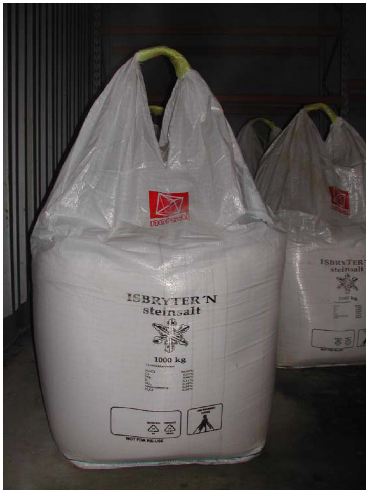
Figur 2.6: Steinsalt levert i storsekk
