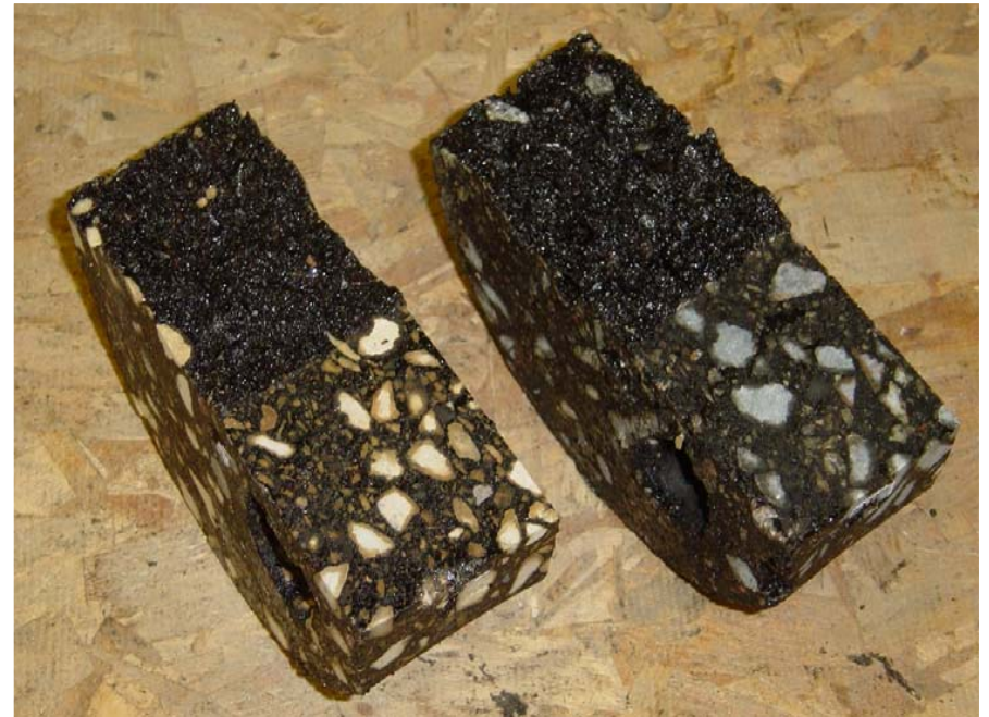
Limestone and granite at high temp
