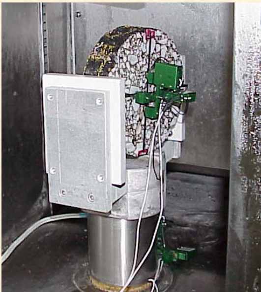
ITT Creep Test - Viscoelastic Properties: D(t,T) and m
