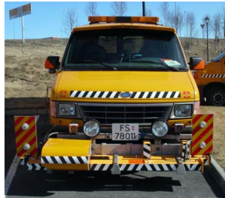
Figure 8: Vehicle "ALFRED" used for measurement of road surface unevenness and texture.
