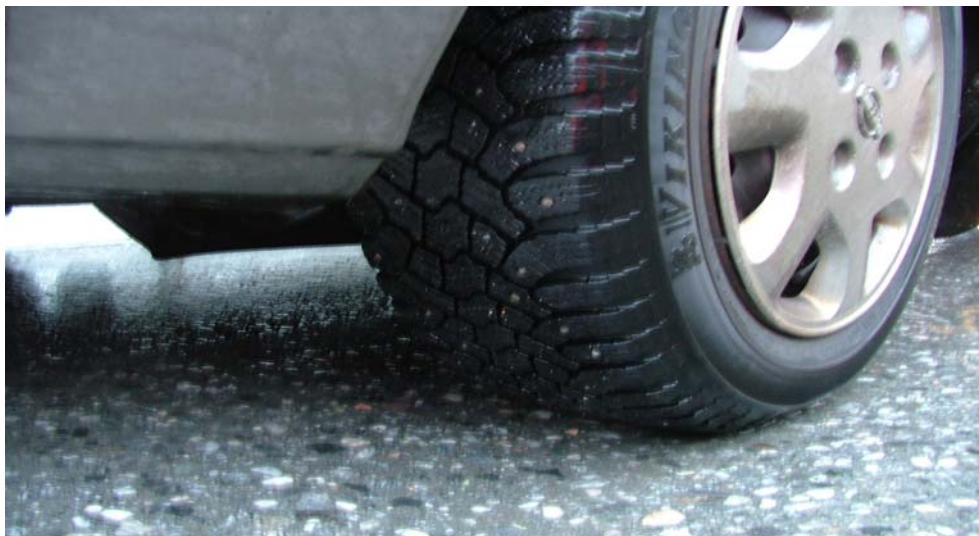
Figure 15: Studded tires, one of the main problems for pavement maintenance.
