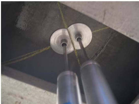
Fig. 5.2 Measurement of central displacement at the bottom side of the panel by the use of two spring loaded displacement transducers (LVDT) with discs on top which can rotate along with the rotation of the panel, as well as bridging over the cracks.
