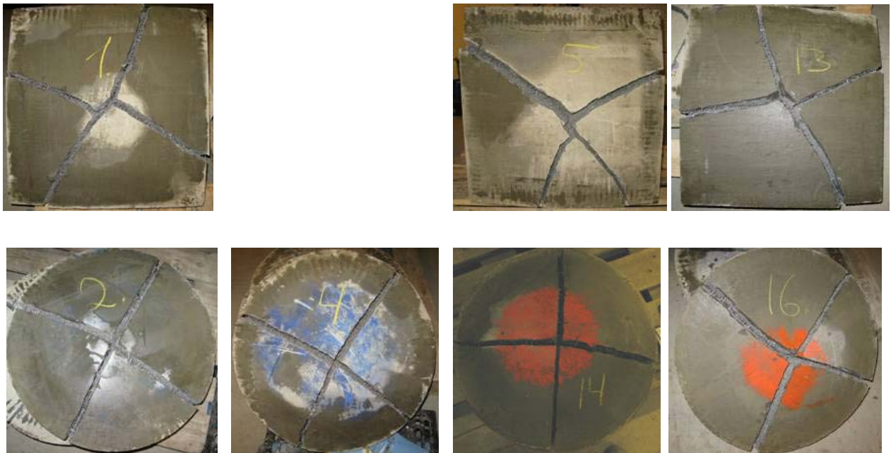
Fig. 6.2 Crack pattern, “no friction” conditions. Square panel no. 3 (“S3”) was not photographed.
