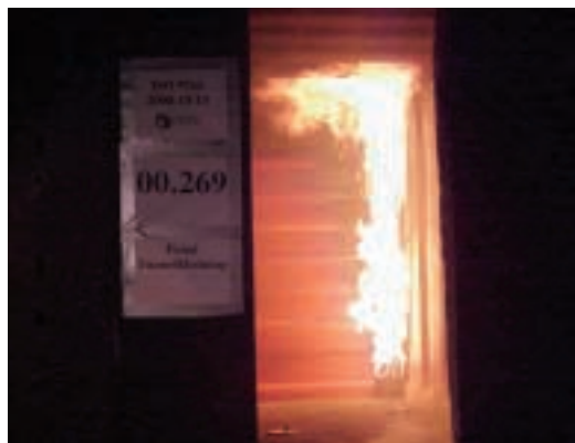
Figur 37 Testing iht. ISO 9705.
