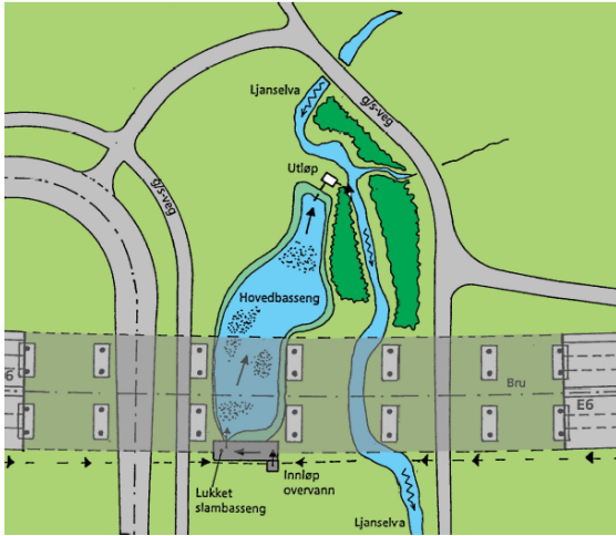
Figure 11: Stormwater pond at E6 Skullerud in Oslo (Norway) with an integral and closed soakaway and water depth of 1.5 m (From Åstebøl and Coward 2005).
