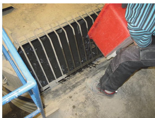
B) Gradually adding fibres while mixing
