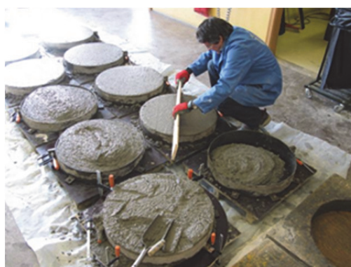
D) Screening of test panels
