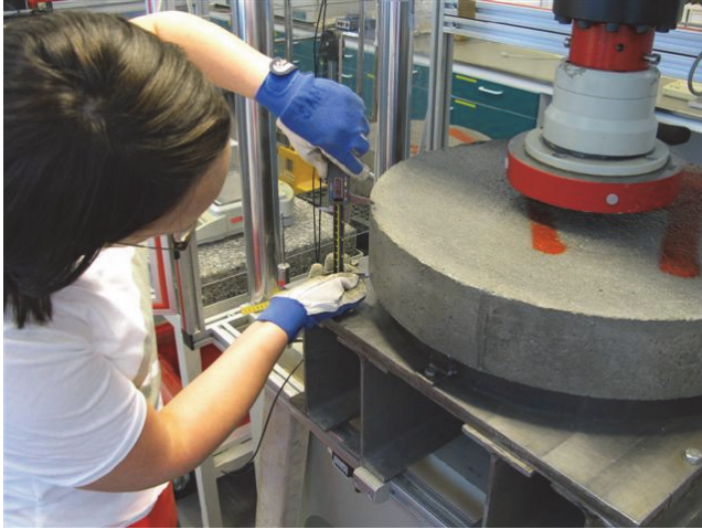
Figure 6 Example of panel thickness measurement with slide gauge
