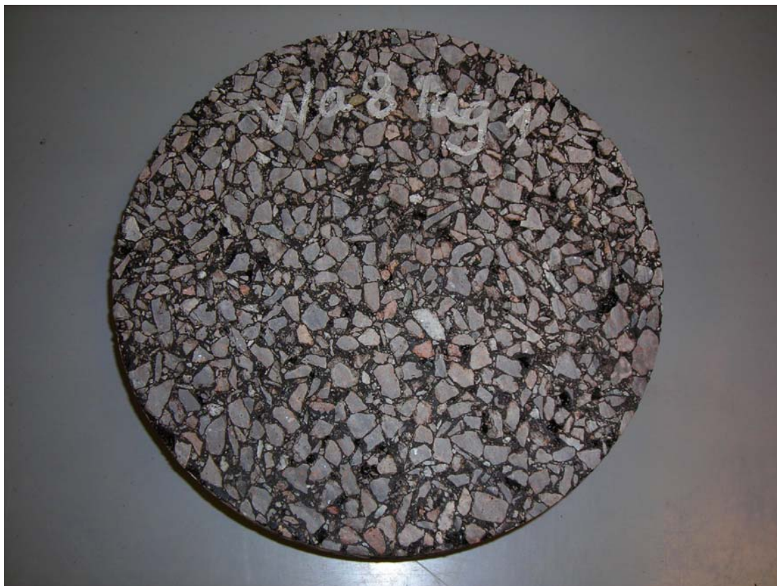
Figur 13 Overflate etter saging for Wa 8
