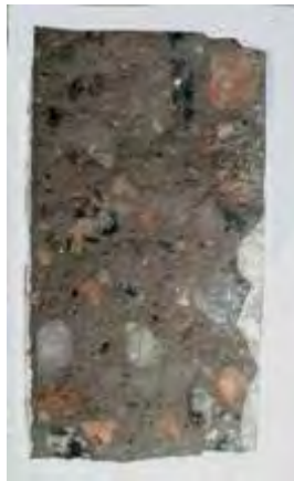
100 % silane, liquid Depth of penetration: 2mm
