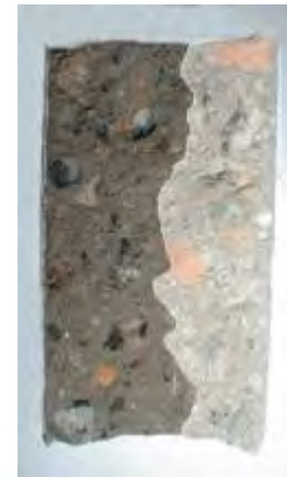
100 % silane, gel Depth of penetration: 22mm
