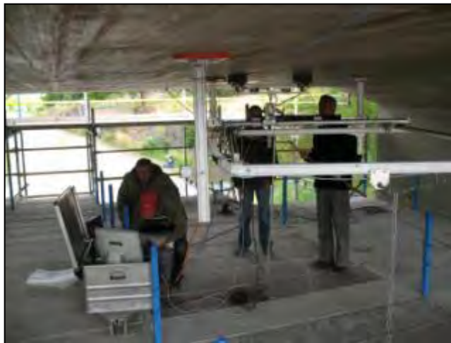
Scanning for steel reinforcement, BAM
