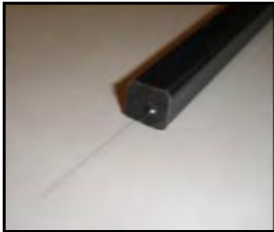
Smart rebar – integrated fibre optic sensors
