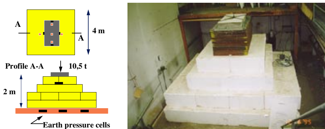
Figure 8: EPS test fill at the Norwegian Road Research Laboratory (now the Road Technology Department)
