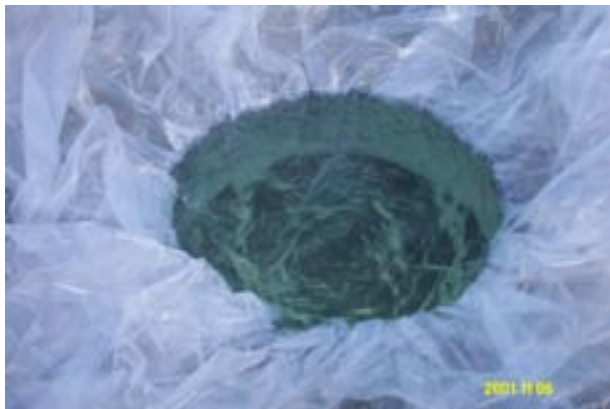
Figure 10: Water used to measure excavated volume.
