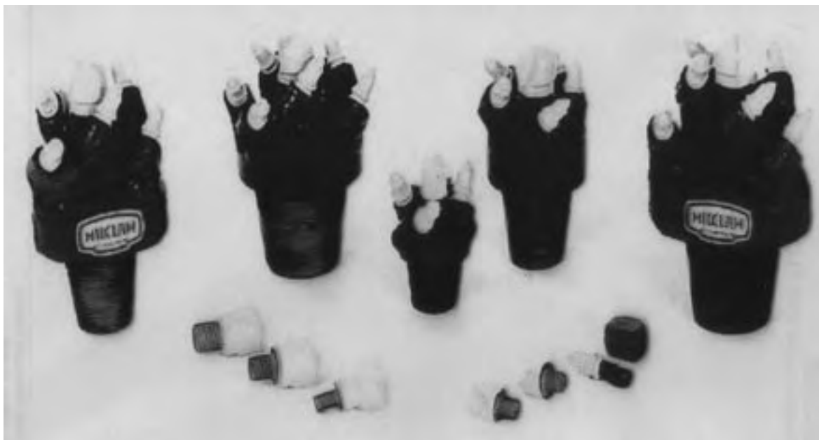
Figure 3: Examples of drill bits with hard-metal, diamond-impregnated cutters.
